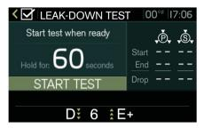
Press and hold the brake pedal until the test is completed.
