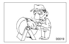
Wear goggles when using a grinder or welder. Pay full attention to safety by wearing gloves when necessary. Watch out for sharp edges, etc. that might injure your hands or fingers.
