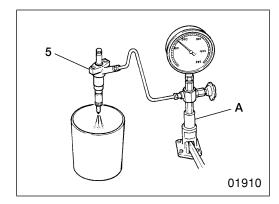
(1) Checking valve opening pressure
