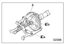
8 Camshaft gear [Removal]
