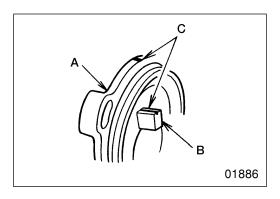
• Align the inscribed lines C on the timer case A and timer B. Then, fit the injection pump assembly 15 onto the air compressor or injection pump drive.
