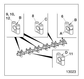
6 8 to 12 14 Installing rocker shaft brackets and rocker shaft Rocker shaft brackets
