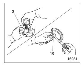
3 10 Impeller-to-water pump shaft interference If the measurement does not conform with the standard value, replace
