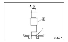
No. 1 idler gear bushing [Removal]
