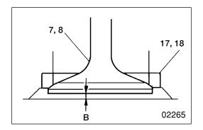
(2) Valve sinkage from cylinder head bottom surface
