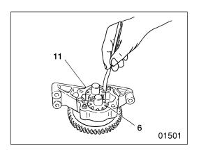
(2) Clearance between gear teeth and case Replace any component whose measurement is out of specification.
