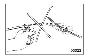
When washing the vehicle, cover the electric system parts and instruments with waterproof material beforehand (Cover with vinyl sheet or the like). Keep water away from harness wire connectors and sensors. If any of them should get wet, wipe them off immediately.
