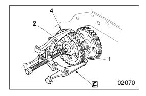
2 4 Removing No. 1 idler shaft and No. 1 idler gear Loosen the bolt 1 by approximately 15 mm (0.591 in.), then remove the No. 1 idler shaft 2 and No. 1 idler gear 4 as a single unit.
