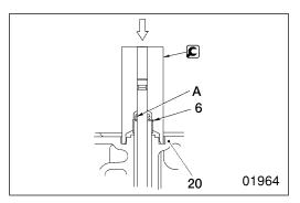
6 Installing valve stem seals
