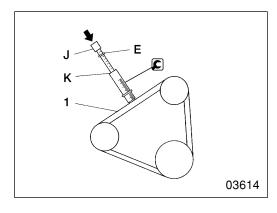
Measure the extent of V-belt 1 deflection A. If the measurement does not conform with the standard value, adjust the V-belt as shown below.
