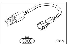
1 Inspecting engine speed sensor
