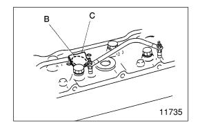
• Cover the injection nozzle mounting hole **B** with a cloth **C**. Then, turn the engine over with the starter and check that no foreign matter adheres to the cloth.
