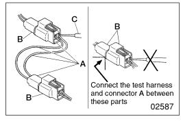
Test with connectors engaged (continuity through circuit obtained) </br><Waterproof connector>
