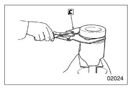
5 to 8 Piston rings and piston Piston rings [Removal]
