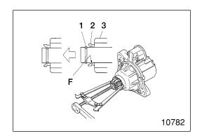
• Pull the pinion 3 strongly to make sure that the stopper ring 1 securely fits in the ring groove F of the pinion stopper 2.
