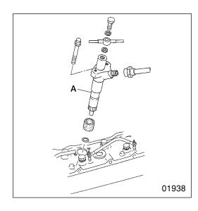
Remove the injection nozzle A.
