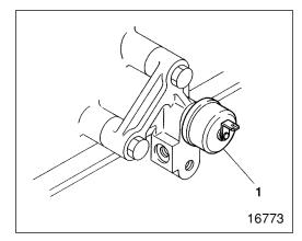
• Remove engine oil pressure gauge unit 1.
