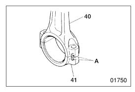
40 41 Installation of connecting rod and connecting-rod cap Align alignment marks A on connecting rod 40 and connecting-rod cap 41.
