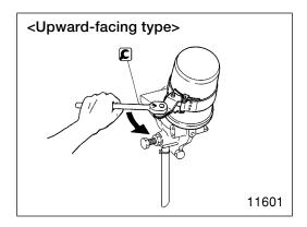
With an upward-facing oil filter, loosen drain plug **1** and air plug **2** in that order, then drain the oil out of filter **3**. [Removal]
