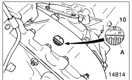
Check that the pointer 10 on the flywheel housing or torsional damper B indicates the value 1° earlier than the correct fuel injection timing.
