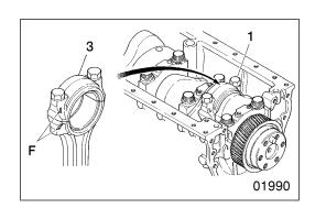
With the piston installed, align the mating marks F on the connecting rod and connecting rod cap 3 and tighten the bolts to the specified torque. Then, tighten the bolts 1 further in accordance with the following procedure.
