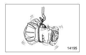
• If you do not have the specified lifting hanger, secure the item using cable taking the point-of-balance of the item into consideration.
