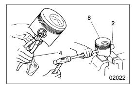
2 4 8 Piston pin, connecting rod, and piston [Removal]
