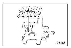
• Do not splash water over the alternator. If water is directly splashed over the alternator, individual components will be short-circuited and might be destroyed.
