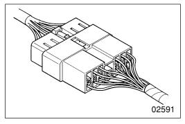
Visual inspection Check for loose connection and poor engagement.
