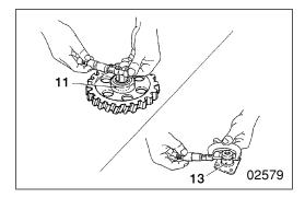
11 13 No. 2 idler gear bushing and No. 2 idler shaft [Inspection]
