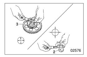
2 3 No. 1 idler shaft and No. 1 idler gear bushing [Inspection]
