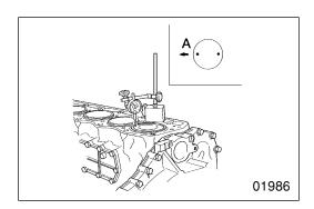
• Measure the projection of each piston at two points and calculate the average of the two values.
