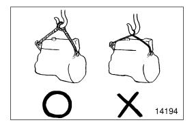
Pay special attention to safety when removing or installing heavy items such as engines, transmissions.
