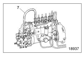
• When the flow of fuel from the injection pipe 7 diminishes, crank the engine more slowly. When the flow of fuel stops completely, stop cranking the engine.
