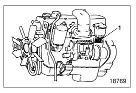
Engine number 1 is punch-marked on the left of the crankcase.
