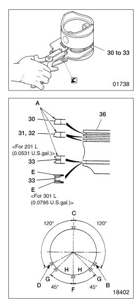
30 to 33 Piston rings [Removal and Installation]
