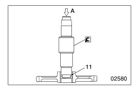
No. 2 idler gear bushing [Removal]
