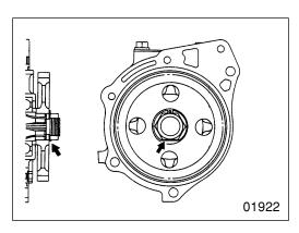
• When the assembly is complete, bend the lock washer 5 down onto the nut 4.
