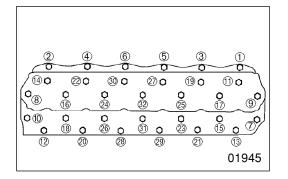
• Loosen and remove the cylinder head bolts 8 in the sequence shown. Each cylinder head bolt should be loosened a little at a time.
