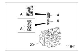
4 5 Installing outer and inner valve springs
