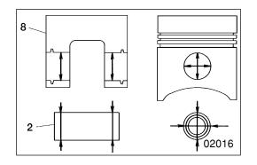
2 8 Piston pin-to-piston clearance
