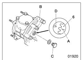
Remove the plug C from the flywheel housing B, then check that the inscribed line A on the drive gear 6 is aligned with the pointer D. If the line and pointer are not aligned, remove and refit the injection pump drive assembly.
