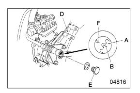
• Remove inspection plug E from flywheel housing D and check that line B on drive gear A is aligned with pointer F. If they are not aligned, reinstall.
