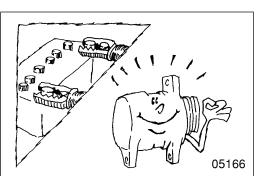
• Disconnect the battery terminals before quick-charging the battery. Quick-charging without disconnecting the battery terminals might damage the diode or regulator.
