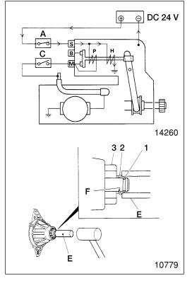
• Immediately (in less than 5 seconds) after the pinion 3 has started rotating, set the switch C to OFF to stop rotation of the pinion.
