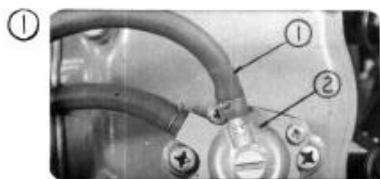
① Fuel tube ② Fuel pump
