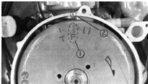
Fig. 29 ① "F" timing mark ② Index mark
