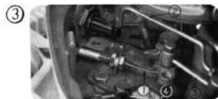
① Throttle cable ② Choke rod ③ Throttle rod ④ Fuel stop rod
