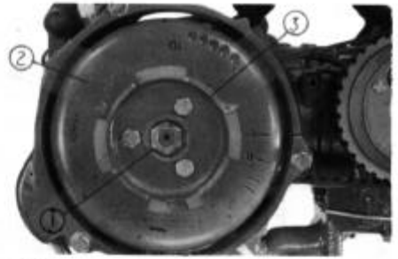
Fig. 27 ① 12mm special nut ② Flywheel ③ Ratchet pulley
