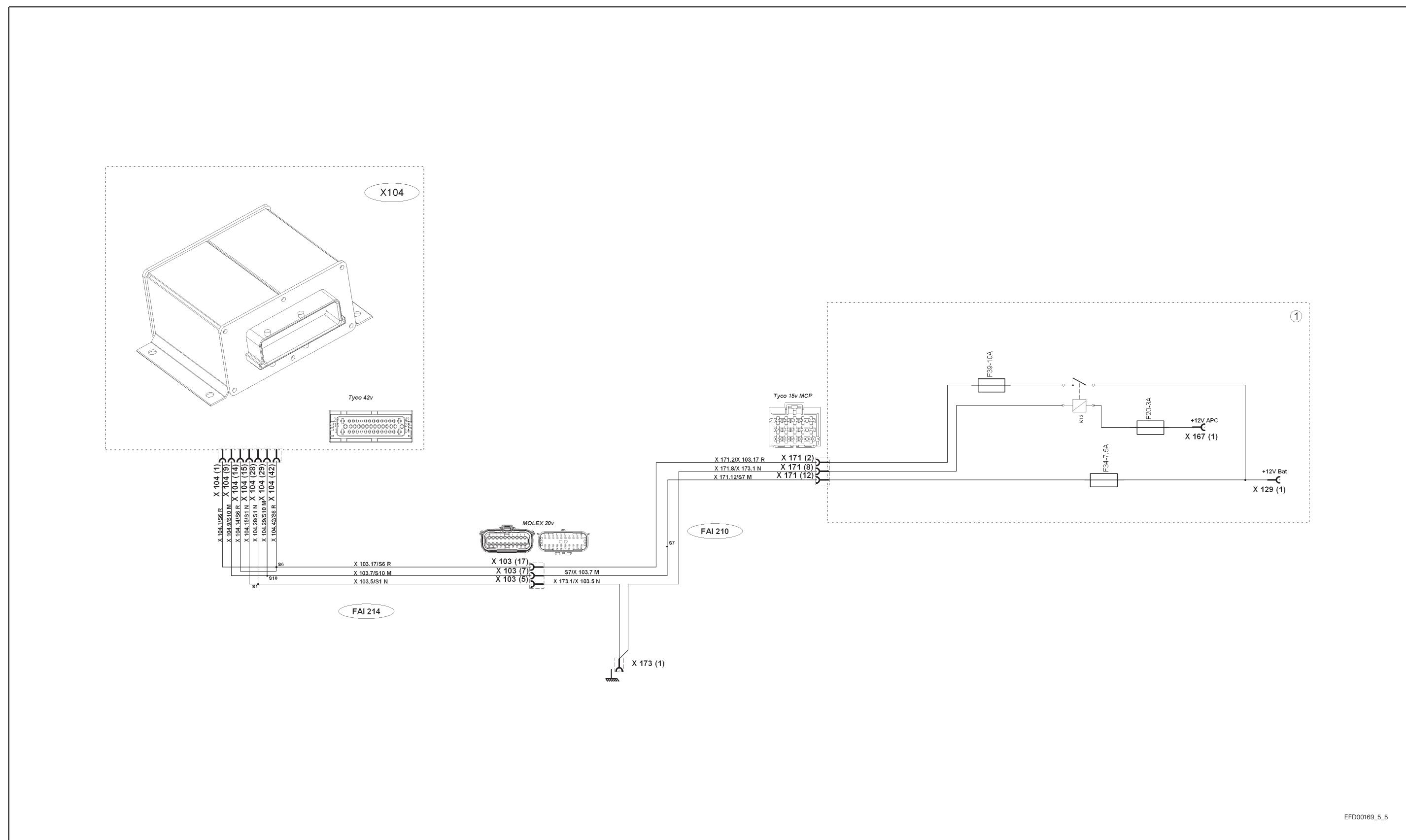
**A.8 Autotronic 5 active suspended cab electrical power supply**
