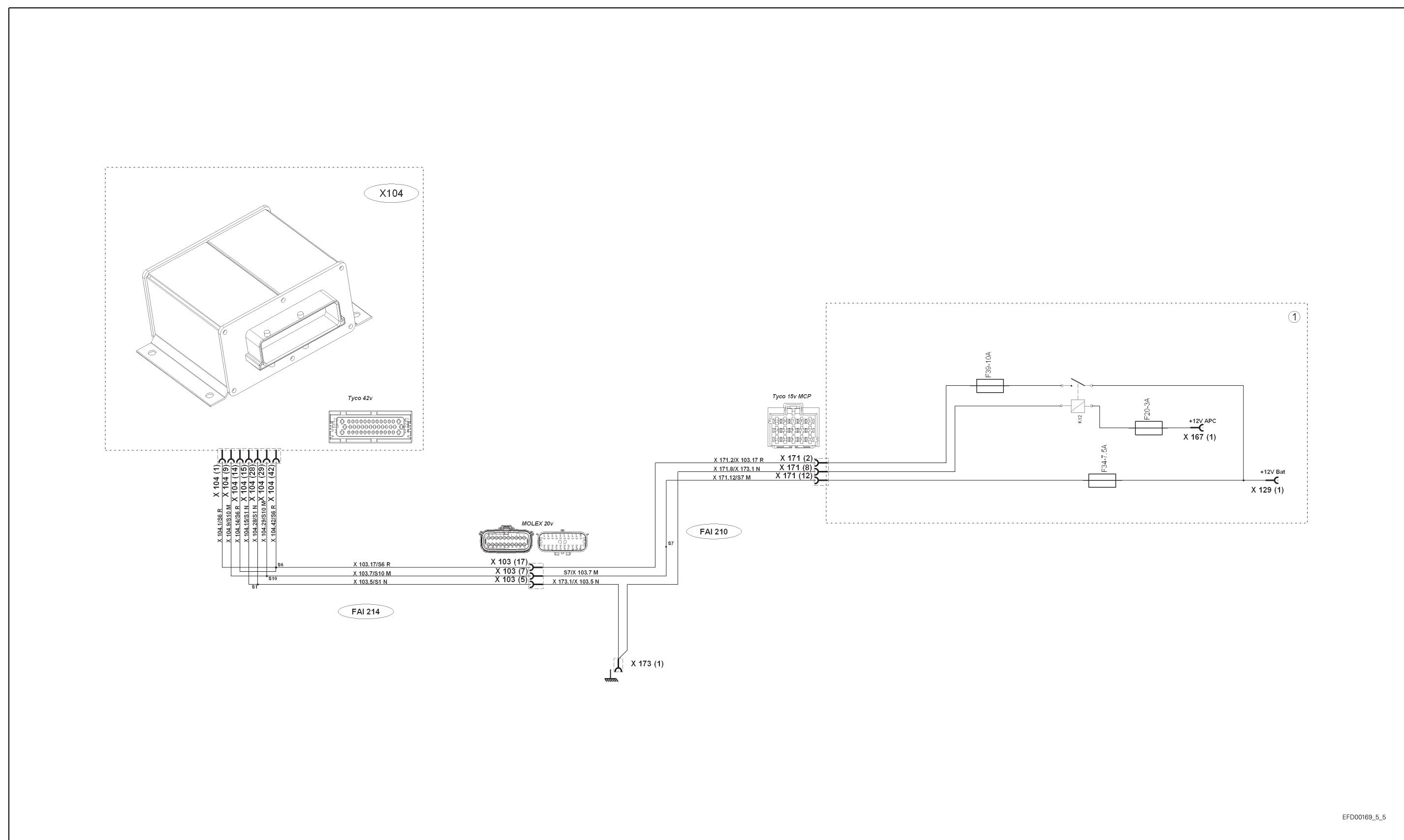
**A.8 Autotronic 5 active suspended cab electrical power supply**
