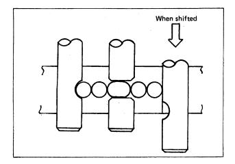
• When a rod is shifted, the inter lock pin(s) is(are) being pushed by the rod, it enters the groove of the neighboringrod, and thus, the inter lock pin locks the rod. Through these operations, the rods other than the shifted rod are locked, preventing double engagement.
