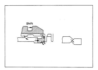
thereby cutting oil film and eases the clutch operation.
