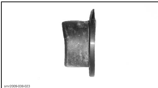
TYPICAL - WORN AND DEFORMED PLASTIC BUSHING
