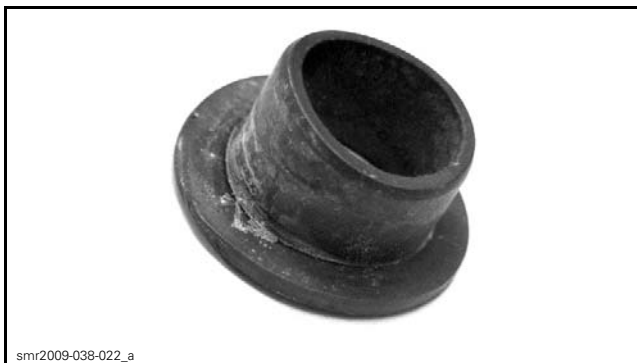
TYPICAL - WORN AND DEFORMED PLASTIC BUSHING
