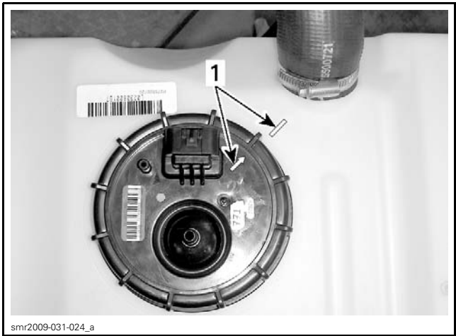
FUEL PUMP MODULE INDEXING 1. Align marks
