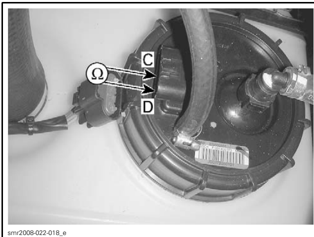
TYPICAL — FUEL LEVEL SENSOR RESISTANCE TEST
