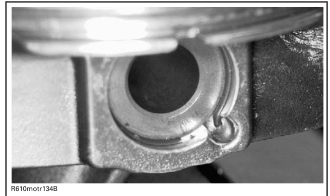
CORRECT POSITION OF THE PISTON CIRCLIP
