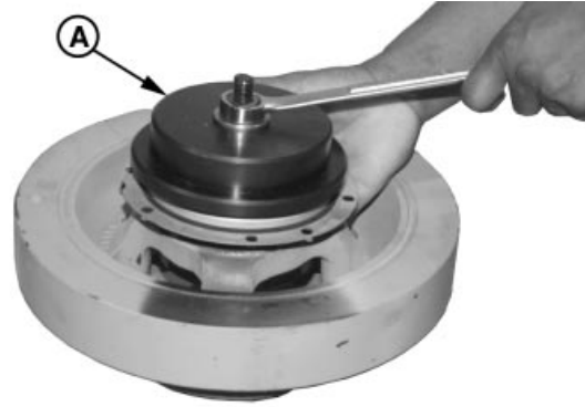
Seating Front Seal on Damper
