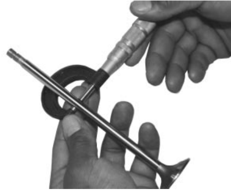
Measuring Valve Stem
