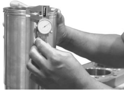
Measuring Liner Flange Thickness
