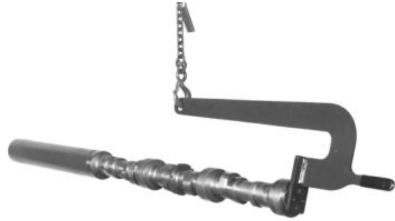
Camshaft with Pilot and Holder
