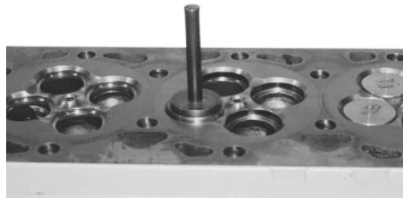
Installing Valve Seat Insert
