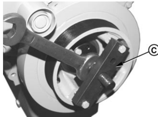
Removing Vibration Damper
