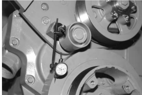
Checking Crankshaft End Play
