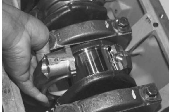
Installing Rod Caps
