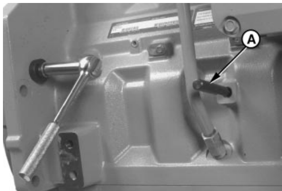
Timing Pin in Crankshaft
