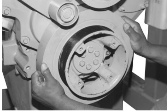
Checking Damper Rotation
