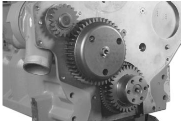
Installing Oil Pump Drive Gear
