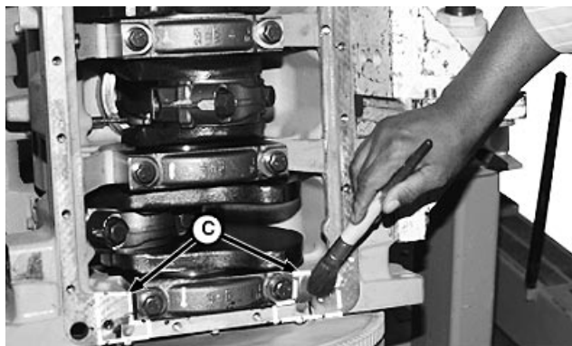
Sealant Applications—Rear Rail
