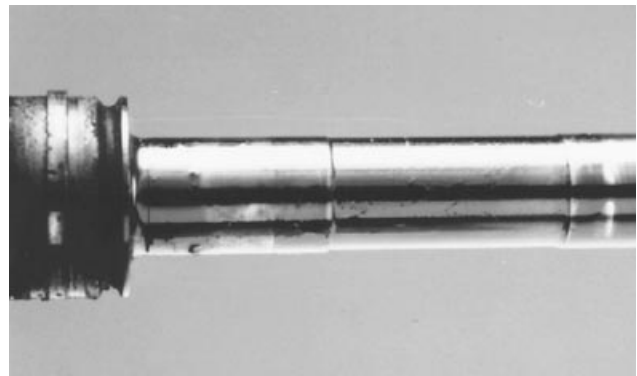
Checking for Oil “Coking” on Shaft
