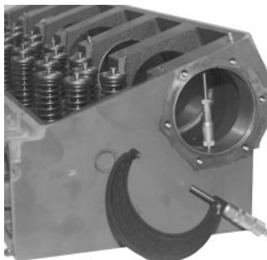
Measuring Camshaft Bushing ID
