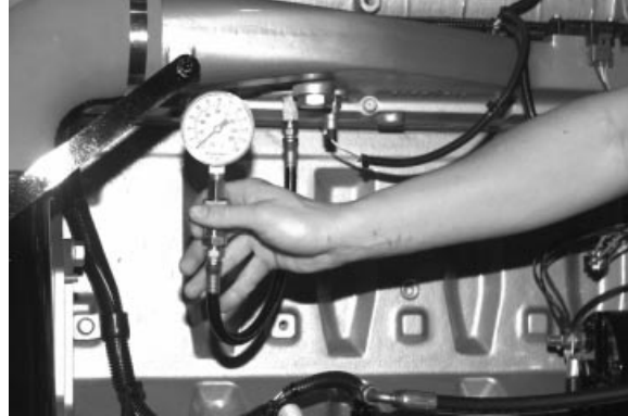
Measuring Intake Manifold Pressure
