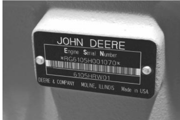
Engine Serial Number Plate
