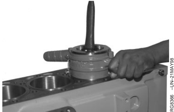
Installing Piston and Rod Assembly
