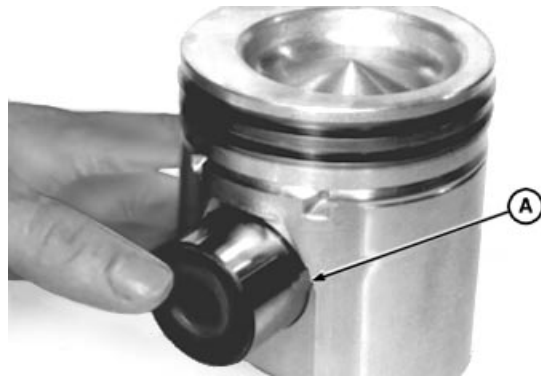
Installing Piston Pin
