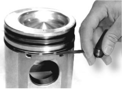
Measuring Oil Control Ring Groove Wear
