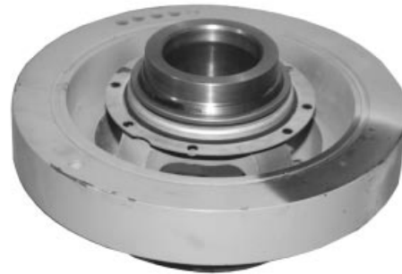
Front Seal Installed on Damper
