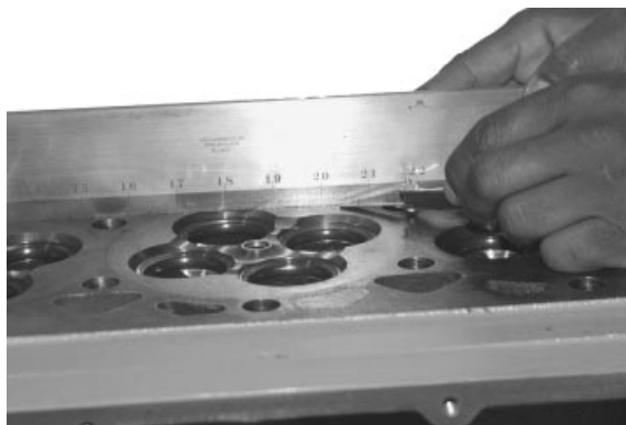
Measuring Cylinder Head Flatness
