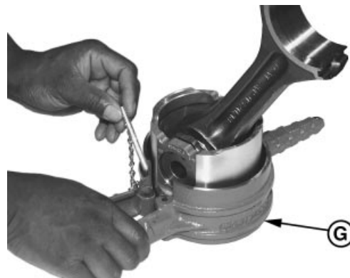
Compressing Piston Rings
