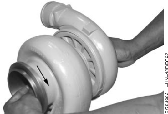
Checking Shaft Rotation and Clearance
