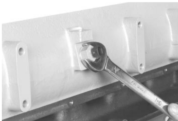
Removing Camshaft Position Sensor
