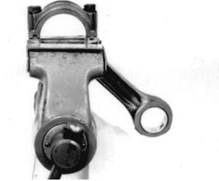
Assembled Rod Without Bearings
