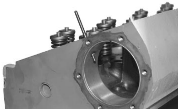
Index Pin Installed through Bushing
