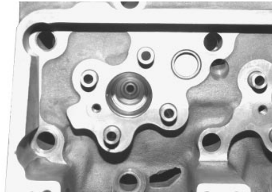
Installed Injector Sleeve
