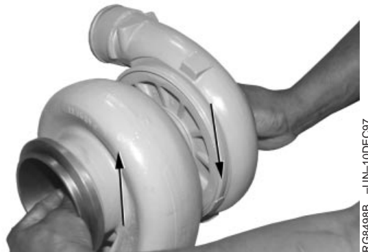
Checking for Contact of Compressor and Turbine Wheels
