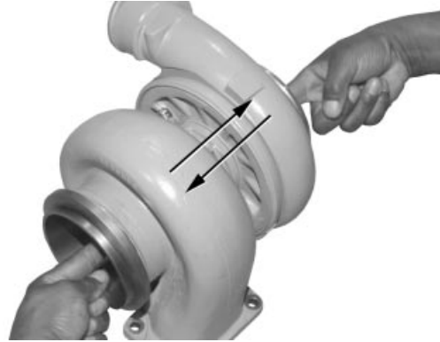
Checking Shaft End Play
