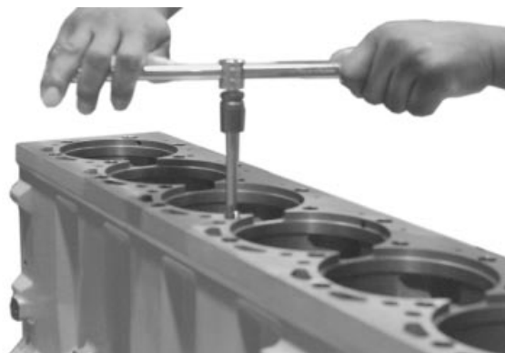
Cleaning Head Bolt Threads in Block
