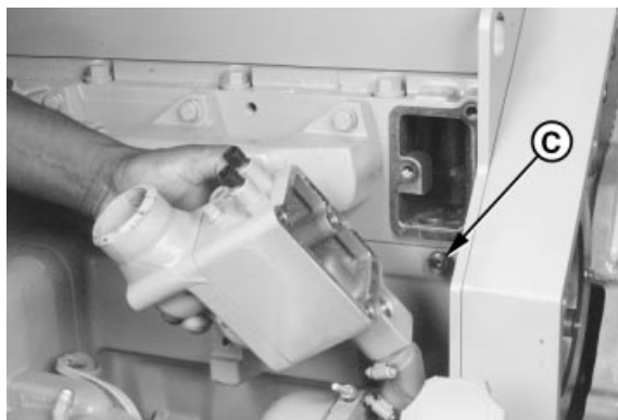
Thermostat Housing Removed
