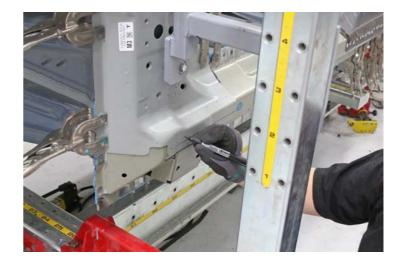
Use a drill with a 6.7 mm (17/64 in) bit to drill holes for structural rivets and countersunk structural rivets.
