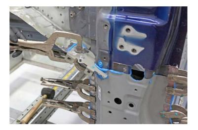
Install the structural rivets and structural countersunk rivets to G install the new Hinge Pillar section and the new A-Pillar to Shotgun Reinforcement.
