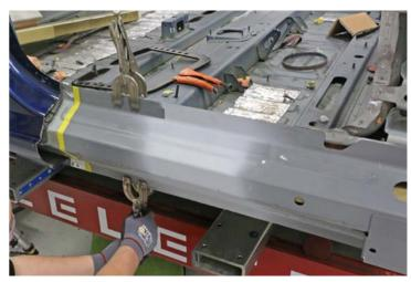
Put the new section into position and clamp it into place. If necessary, trim the new section to fit.
