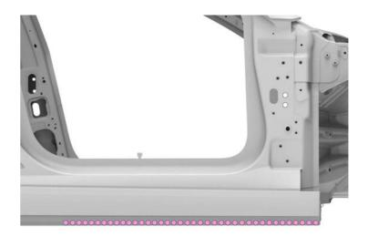
Install the structural rivets and structural countersunk rivets.
