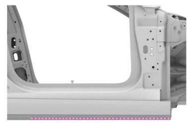
Use a drill with a 6.7 mm (17/64 in) bit to drill holes for structural rivets and structural countersunk rivets.
