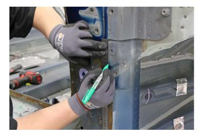
Cut the original Hinge Pillar on the cut lines marked in the previous substep.
