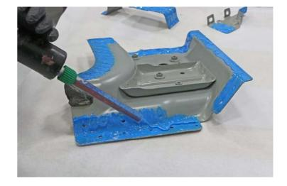
Install the new Hinge Pillar Assembly section.
