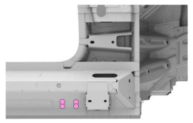
Use a drill with a 6.7 mm (17/64 in) bit to drill holes for structural rivets through the holes in the template, and then remove the template.
