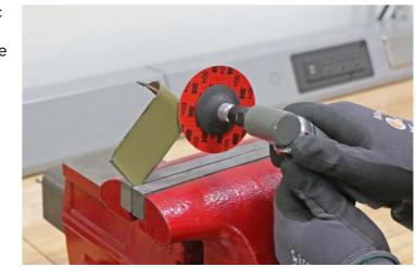
Use a disc sander with a medium-abrasive surface conditioning disc to remove the e-coat on the outward surface of the backing plates (the sides of the backing plates that will be facing the outside of the vehicle when installed).
