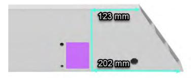
Use a red Scotch-Brite pad or equivalent to scuff each of the new Sill Insert Mounting Brackets in the bond path area.
