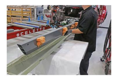
Mark holes for structural rivets on the new Sill Outer Assembly. Structural Rivet, 6.5 mm Short (x8)
