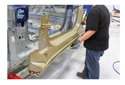
Create and install backing plates for the Body Side Outer butt joints.
