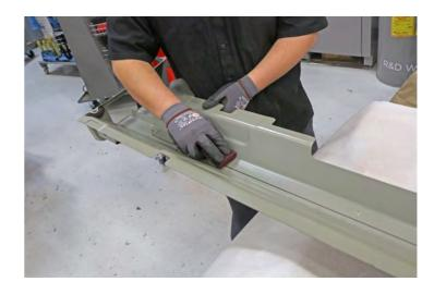
Clean all the bond paths on the new Sill Insert and the new Sill Outer Assembly with isopropyl alcohol (IPA).
