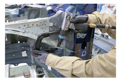
Use a hammer and chisel to remove the A-Pillar to Shotgun Reinforcement.
