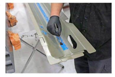
While the primer layer is still wet, apply a bead of structural adhesive on top of the primer layer on the new Sill Outer Assembly.
