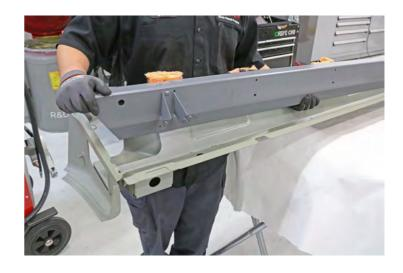
Use a red Scotch-Brite pad or equivalent to scuff the new Sill Insert and the new Sill Outer Assembly in the bond path areas.
