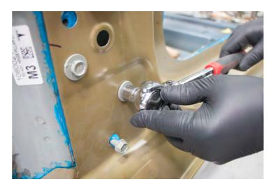
Insert the structural rivets and the structural countersunk rivets. O Structural Countersunk Rivet, 6.5 mm (x2, circled in red) Structural Rivet, 6.5 mm Short (x78)
