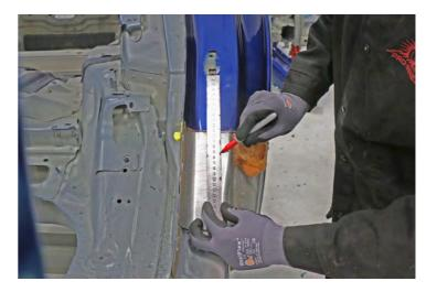
Cut the aluminum C-Pillar Extension on the cut line marked in the previous substep.
