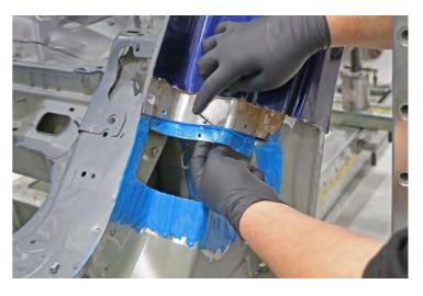
Put the new C-Pillar Extension section into position and insert the structural rivets and countersunk rivets to hold it in place.
