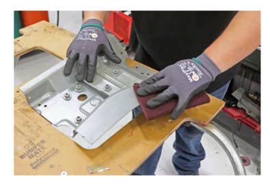
Mark the installation spot weld locations on the new Hinge Pillar Assembly section, the A-Pillar to Shotgun Reinforcement, and the vehicle.
