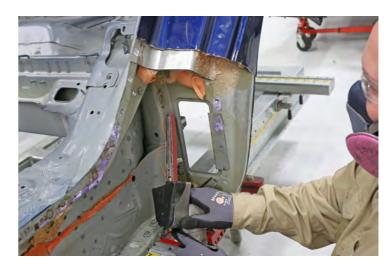
Remove the seam sealer in the area of the factory self-piercing rivets.
