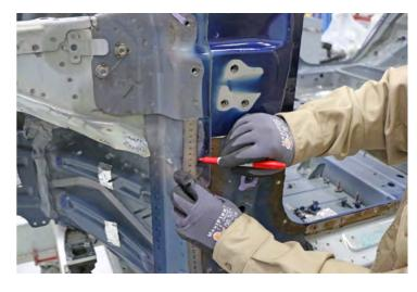
Cut the Hinge Pillar on the cut lines marked in the previous substeps.
