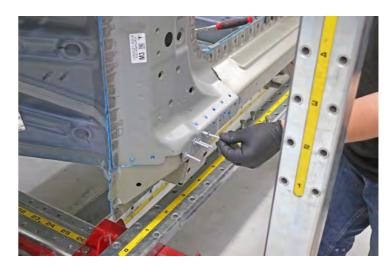
Install the structural countersunk rivet shown. O Structural Countersunk Rivet, 6.5 mm (x1)
