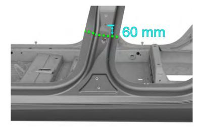
Mark a cut line in the C-Pillar area 110 mm (1-9/16 in) down from the lower edge of the bolt hole shown.
