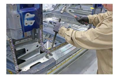
Mark a cut line on the original Sill Insert. Cut Line
