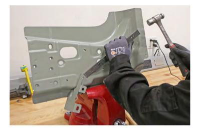
Cut the second new Hinge Pillar Assembly on the green dashed line shown.
