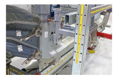
Put the new A-Pillar to Shotgun Reinforcement into position and insert grip screws into the holes that were drilled when the reinforcement was removed in an earlier substep.
