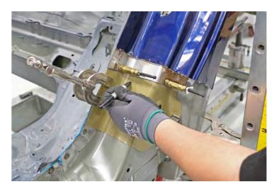
Use a drill with a 4.8 mm (3/16 in) bit to drill holes for structural rivets and countersunk structural rivets.
