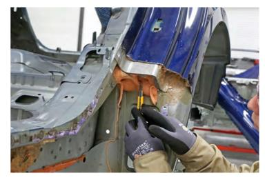
Use a drill with a spot weld bit to drill out the spot welds shown.
