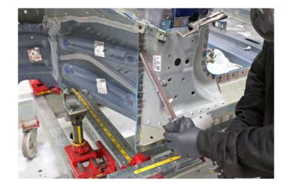
Bake the structural adhesive so that the bonded panels reach a temperature of 60°C-80°C (140°F-176°F) for at least 30 minutes to achieve full strength.
