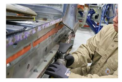
Use a heat gun to heat the adhesive joints, and then use a hammer and chisel to remove the remaining piece of the middle portion of the Sill Outer Assembly where it meets the B-Pillar Outer.
