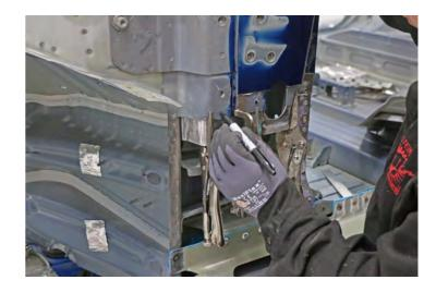
Use a drill with a 6.7 mm (17/64 in) bit to drill holes for structural countersunk rivets.
