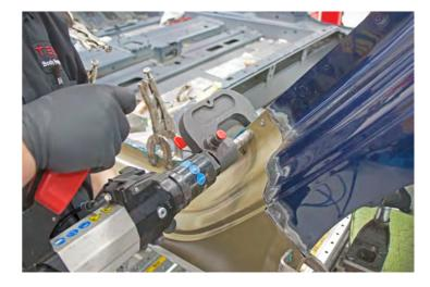
If the Sill Outer was attached to the Sill Inner with resistance spot welds: Clamp the lower flange area until the structural adhesive cures.
