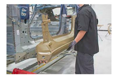
Mark the bond path and weld areas on the new component and the vehicle. These areas will be prepared for bonding and welding in the next step.
