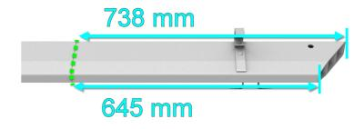
Cut the new Sill Reinforcement on the cut line marked in the previous step.
