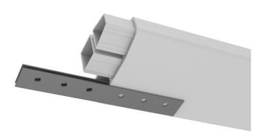
Use the existing holes on the reinforcement plates as a guide to drill 8 mm holes for hex-head bolts in the Sill Insert Section.
