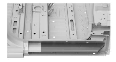
Adjust the front of the new Sill Insert front section so that it is 114 mm from the bottom edge of the Sill Inner lower flange.
