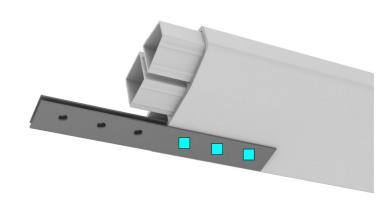
Position the new Sill Insert front section on the vehicle and clamp it into place.
