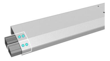
Position inner and outer reinforcement plates on the new Sill Insert front section and loosely install the bolts to hold it in place.
