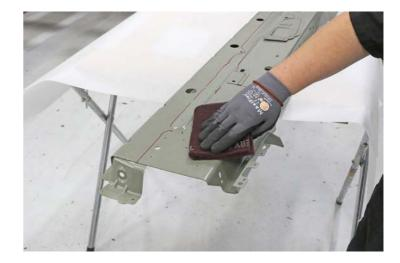
Use a disc sander with a medium-abrasive surface conditioning disc to remove the e-coat on the new component and on the vehicle in the weld areas. Use a belt sander with a medium-abrasive belt for any areas that cannot be reached with a disc sander.
