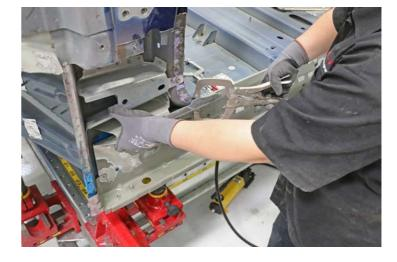
Align and temporarily secure the new component to the frame bench jig points.
