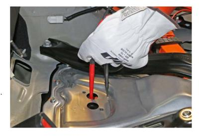
Remove the High Voltage Battery (Service Manual procedure 16010101).
