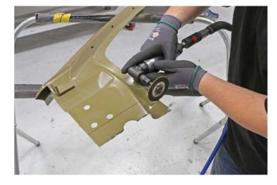
Partial Trim the excess material from each section to match the backing plates shown.
