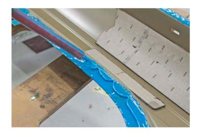
12 Install the new Body Side Outer section.
