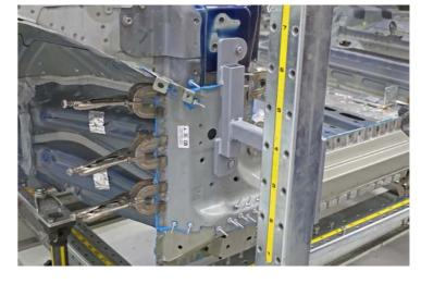
Clamp the new Hinge Pillar section and the A-Pillar to Shotgun Reinforcement in the areas that do not have fasteners.
