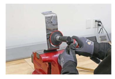
Put the backing plate into position and clamp it into place.
