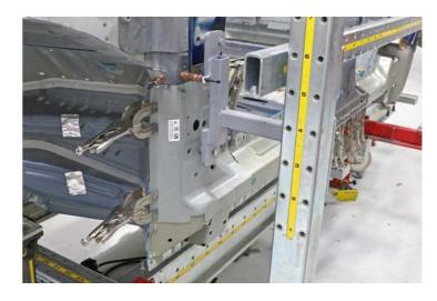
Put the new A-Pillar to Shotgun Reinforcement into position and insert grip screws into the holes that were drilled when the reinforcement was removed in an earlier substep.
