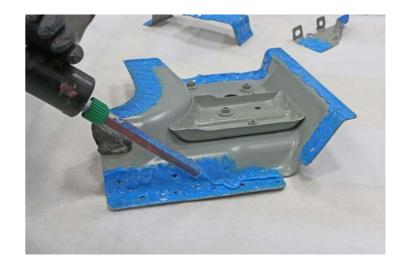
Install the new Hinge Pillar Assembly section.
