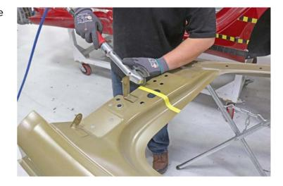
Put the new Body Side Outer section into position and check for suitable gaps. If necessary, trim the new Body Side Outer section. Remove the new Body Side Outer section.
