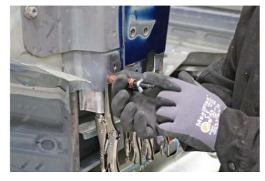
Use a drill with the Microstop countersink cage assembly and the appropriate-sized countersink bit to countersink the holes for countersunk rivets (Microstop Countersink Kit, Tesla p/n 1133101-00-A).
