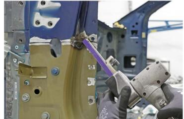
Secure the butt joint flanges.
