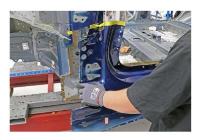
**?** Remove the lower portion of the Hinge Pillar.
