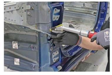
Use a drill with a spot weld bit to drill out the spot welds that attach the lower portion of the Body Side Outer.
