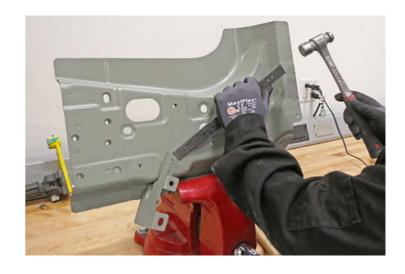
Cut the first new Hinge Pillar Assembly as shown to create a backing plate.
