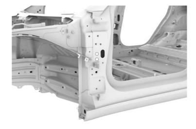
Install the structural countersunk rivets.
