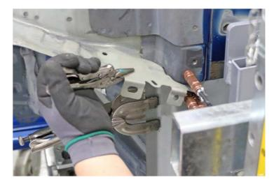
Mark the remaining fastener locations on the new Hinge Pillar Assembly section.
