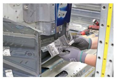
Mark the bond path areas on the new Hinge Pillar Assembly section, the new A-Pillar to Shotgun Reinforcement, the backing plate, and the vehicle.
