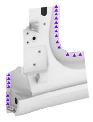
Use a disc sander with a medium-abrasive surface conditioning disc to remove the e-coat in the GMA weld and installation spot weld areas.
