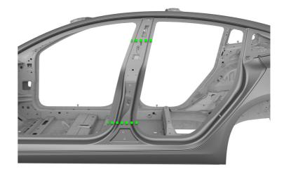
Mark cut lines at the top of the front door opening 200 mm to the rear of the roof rack bracket shown and 10 mm to the rear of the roof rack bracket shown.
