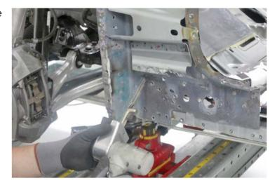
Use a heat gun to heat the adhesive joints, and then use a hammer and chisel to remove the remaining pieces of the original component.
