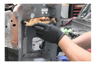
Seal the seams in the factory locations, and as necessary.
