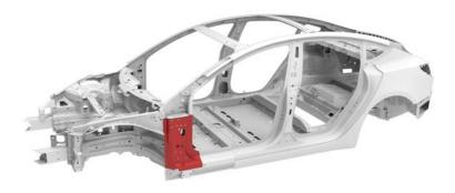
Remove the Sill Inner (Front Section).
