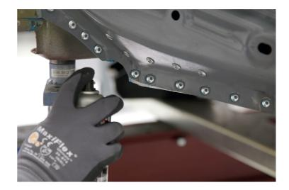
After refinishing, use a 360-degree spray wand of suitable length to apply corrosion-proofing material on the inside of the enclosed area to
