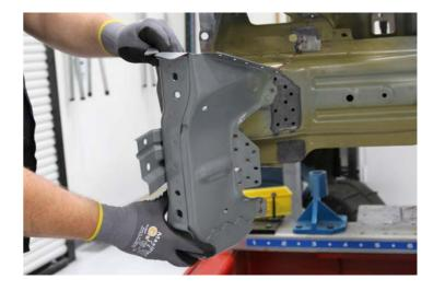
Use a drill with a 10 mm (13/32 in) bit to drill holes for plug welds in the new component.
