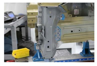
Install 2 of the original crush can bolts and the bolt that attaches the Shotgun Tower to the Front Frame Rail Inner, but do not torque them fully at this time.
