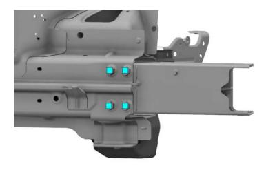
Install the new Fender and Lamp Support Bracket.
