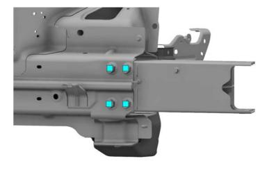
Remove the crush can.
