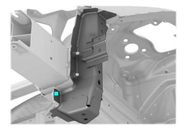
Mark cut lines to prepare to cut away the bulk of the original component.
