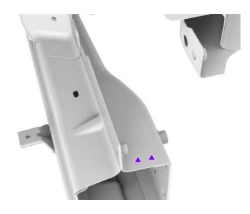
Use a disc sander with a medium-abrasive surface conditioning disc to remove the e-coat on the new component and on the vehicle in the weld areas. Use a belt sander with a medium-abrasive belt for any areas that cannot be reached with a disc sander.
