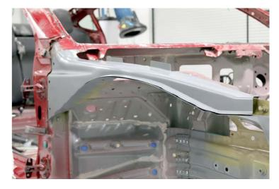
Insert the 3 bolts that were removed in an earlier substep, but do not torque them fully at this time.
