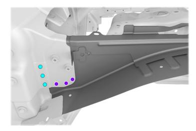
Install the structural bulb rivets and structural rivets.
