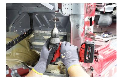
Mark the vehicle and the new component in the areas that need to С have e-coat removed.
