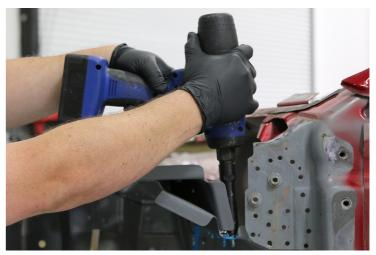
Install the structural bulb rivets and the structural rivet.
