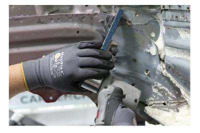
Use a hammer and chisel to remove the remaining pieces of the component.
