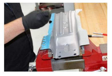
While the primer layer is still wet, apply a bead of structural adhesive on top of the primer layer on the vehicle.
