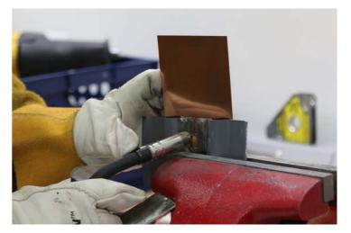
Use a disc sander to grind down the weld.
