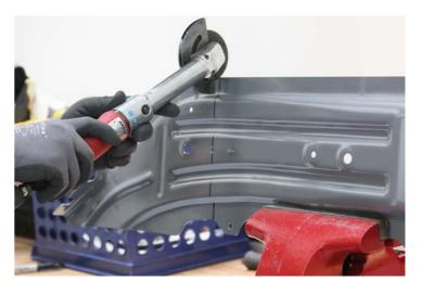
Put the new section into position and align it to the frame bench jig point.
