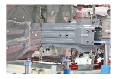
2 Create a reinforcement plate to reinforce the joined sections of the Front Frame Rail Outer.
