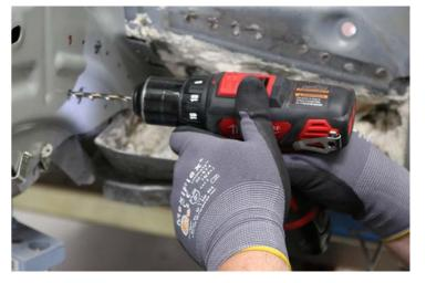
Use a drill with the Microstop countersink cage assembly and the appropriate-sized countersink bit to countersink the hole (Microstop Countersink Kit, Tesla p/n 1133101-00-A).
