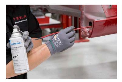
After refinishing, use a 360-degree spray wand of suitable length to apply corrosion-proofing material on the inside of the enclosed area to prevent corrosion.
