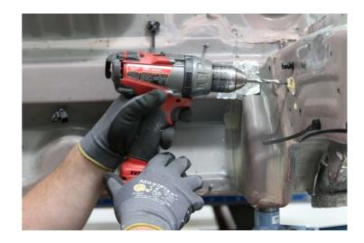
Use a drill with a spot weld bit to drill out the factory spot welds.
