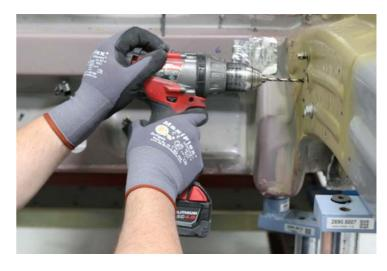
Use a drill with a 6.7 mm (17/64 in) bit to drill holes for the structural rivets shown.
