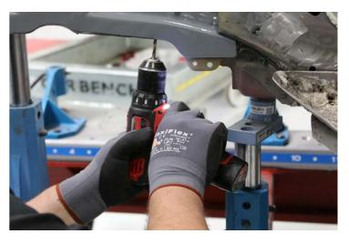
Mark the installation spot weld locations on the new component and the vehicle.
