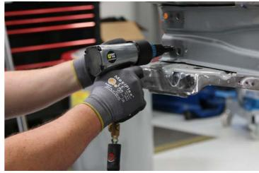
Use a heat gun to heat the adhesive joints, and then use a hammer and chisel to remove the original component.
