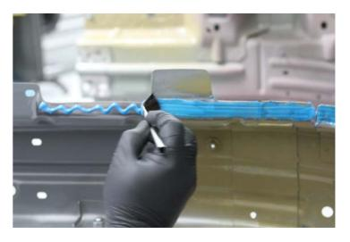
While the primer layer is still wet, apply a bead of structural adhesive on top of the primer layer on the vehicle.
