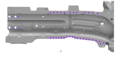
Use a disc sander with a medium-abrasive surface conditioning disc to remove the e-coat on the new component and on the vehicle in the weld areas. Use a belt sander with a medium-abrasive belt for any areas that cannot be reached with a disc sander.
