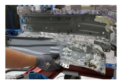
Remove any remaining structural foam.
