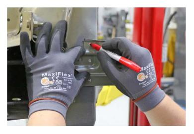
Mark the bond path areas on the new component and the vehicle. These areas will be prepared for bonding in the next step.
