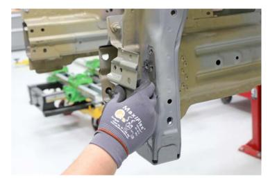
Use a drill with a 6.7 mm (17/64 in) bit to drill a hole for a structural bulb rivet on the vehicle.
