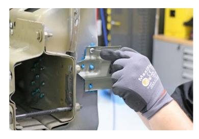
Install the structural bulb rivets.
