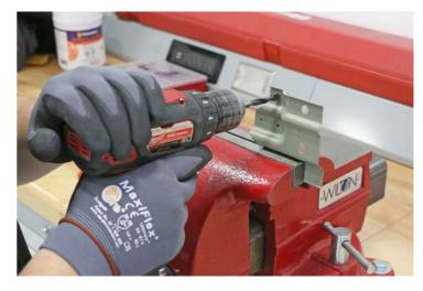
Put the new component into position and mark the structural bulb rivet locations on the vehicle.
