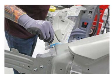
Clamp the new section or sections into place.
