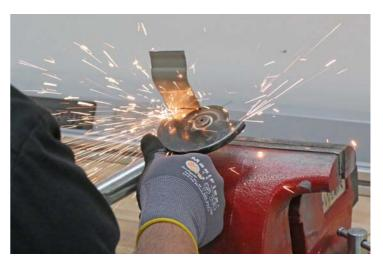
Put the backing plates into position and check their fit. If necessary, trim them to fit.
