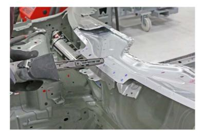
Clean the plug weld areas on the new section and on the vehicle with isopropyl alcohol (IPA).
