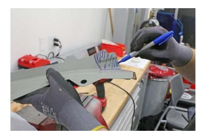
If replacing the middle section: Use a drill with an 8 mm (5/16 in) bit to drill holes for plug welds in the new section.
