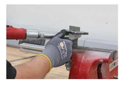
Cut the backing plate down the middle to create 2 backing plates.
