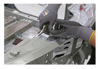
Mark the backing plates in the butt joint weld area.
