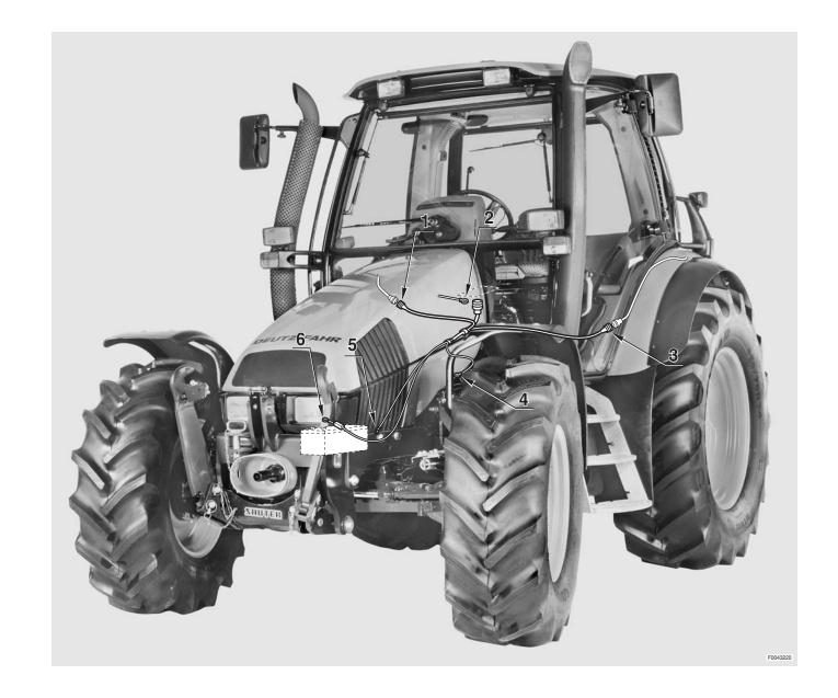
FRONT AXLE SUSPENSION WIRING 0.012.8673.4
