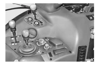
2 - Disconnect the control cable (1) from the control lever(2) and remove the yoke (3) to remove the outer cable(4).
