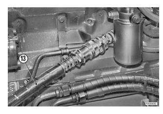
10 - Unplug the connector and remove the air conditioning compressor (14).
