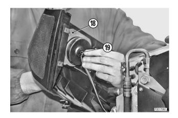
4 - Remove the lamp assemblies (18) by rotating them to the rear and moving them sideways to disengage the release button (8).
