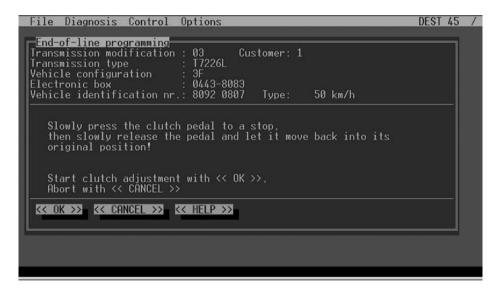
Fig. 39 - Clutch adjustment
