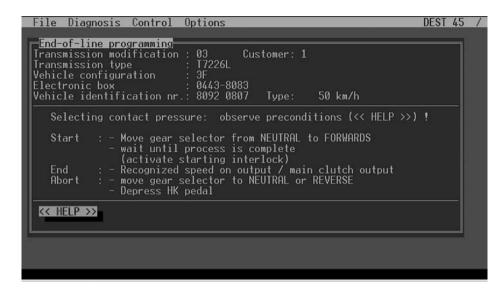
Fig. 40 - Determination of contact pressure
