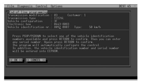
Fig. 38 - Select vehicle identification number
