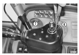
5 - Lift off the switch unit (7) and place it to one side.
