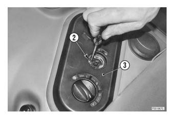
3 - Detach the control panel (3) by pressing the spring clips (4) securing it to the left-hand console.
