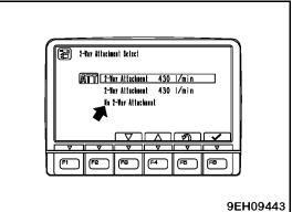
On the working mode selection screen, it is not possible to select No 2-Way Attachment.
