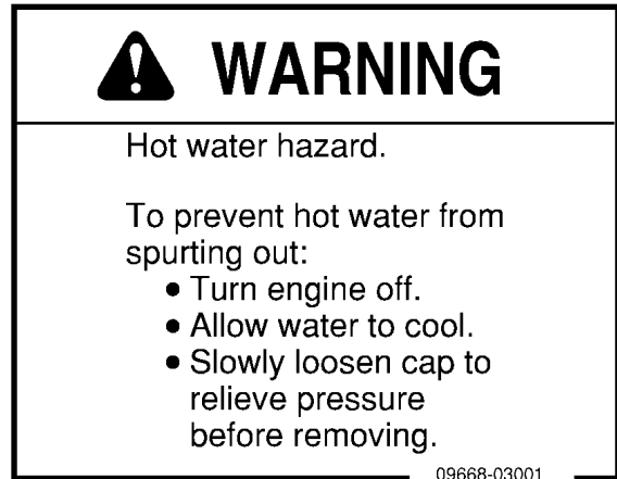
(16) Precautions for high-temperature cooling water (09668-03001)
