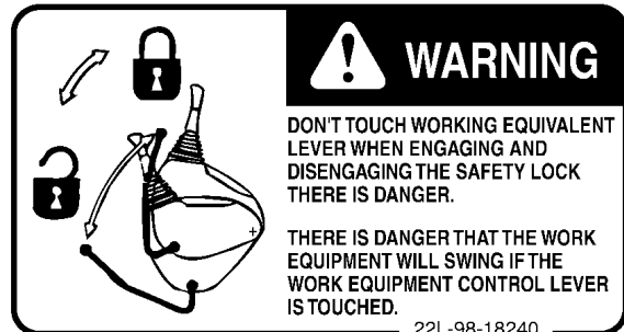
(10) The safety lock is operated with the lock lever (22L-98-18240)
