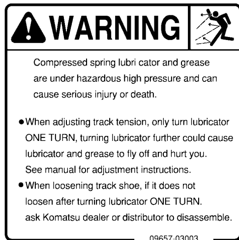
(18) Precautions for checking and adjusting track tension (09657-03003)
