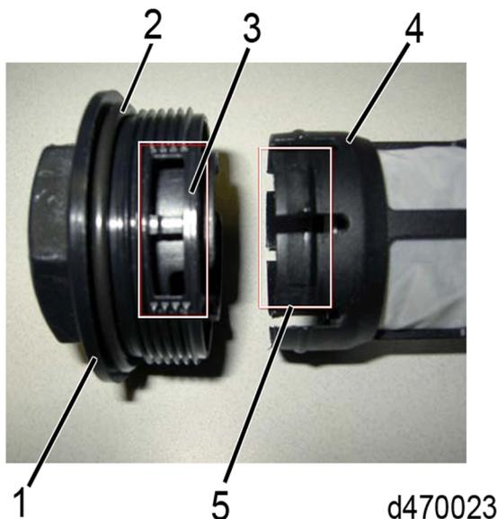
2. Apply a thin coat of petroleum-based lithium grease to the prefilter cap seal ring (2).
