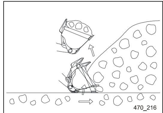
8. If there is too much material inside the bucket, you must briefly tip it in, dump it and lower it in order to reduce the load and to prevent that you lose the load during the transport.
