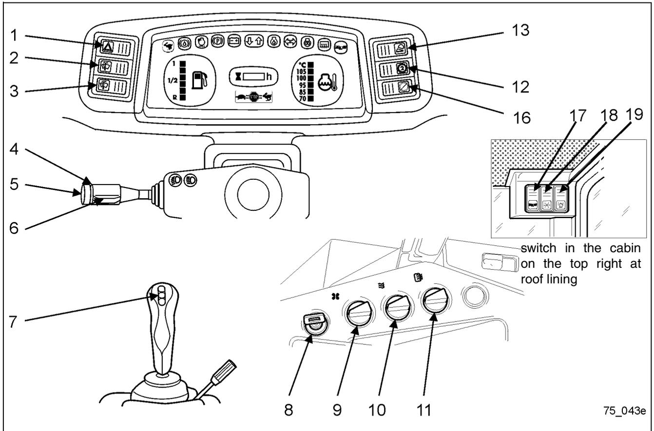
1. Switch and control lamp of hazard flashers
