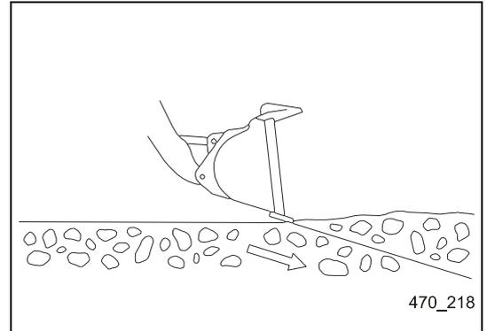
4. While driving forward, move slightly the multi-function lever of the boom in order to remove only a thin layer of the surface of the soil to be removed.
