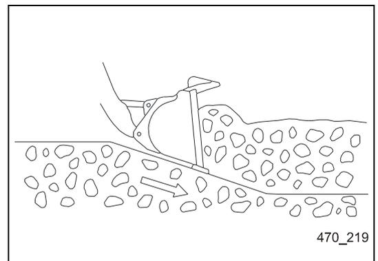
5. Move the multi-function lever of the boom slightly up and down to reduce the resistance during driving forward. While removing, ensure that the digging force is not applied only on one side of the bucket.
