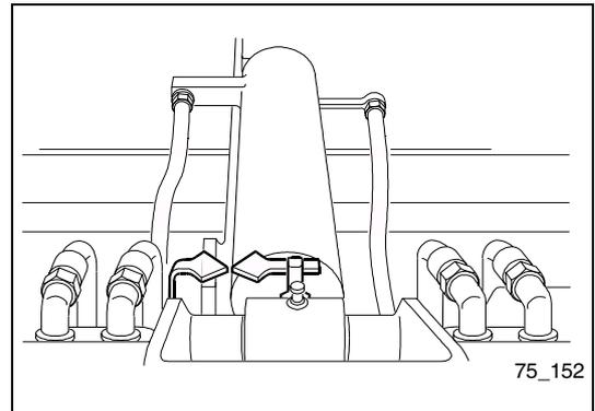
3. Turn the lock lever for the work unit to position '1'. The boom will then be blocked during rides on public roads and cannot be moved.
