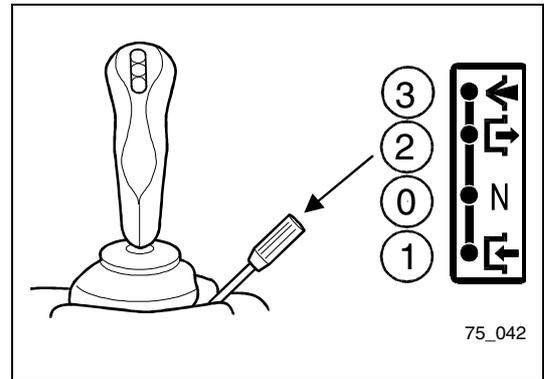
If the multi-purpose bucket is attached to the quick-change unit, the control lever has the functional assignment described above. If the switching lever for the bucket is in position '1', the multi-purpose bucket is active. You can then operate the multi-purpose bucket via the control lever for special equipment. It then has the following functions:
