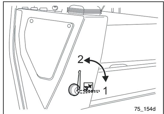
5. Release the parking brake. Press the celebration adjustment knob to this at the parking brake lever. Press down the locking button of the parking brake lever. Then, release the locking button. The parking brake warning light goes out.
