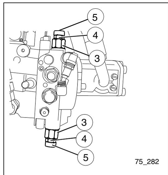
After towing another machine loosen the counter-nut (4) and the threaded stud (5) by turning it anti-clockwise until it reaches the limit stop. Hold the valve (3) in position using a wrench and re-tighten firmly the counter-nut (4). Perform these operations on both valves.
