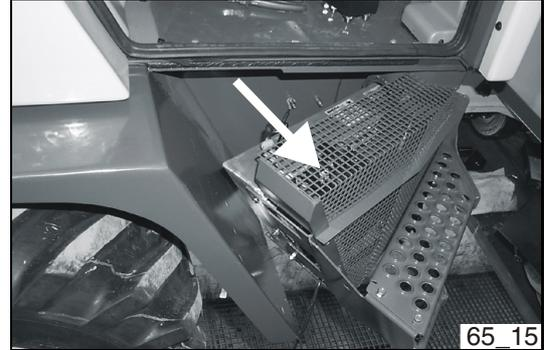
Operate the cooler of the air-conditioning system for 5 - 10 minutes, then touch the high pressure portion and low pressure portion of the compressor (or high pressure hose and low pressure hose joint) with your hand. At the same time, inspect the flow of coolant (R134a) through the sight glass to check the gas level.
