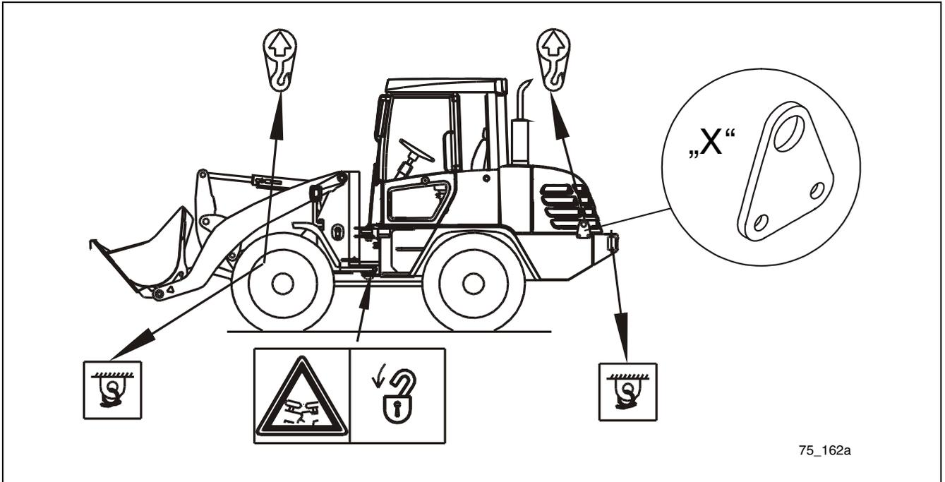
Information signs attached to the machine indicate the attachment points. To avoid damage to the machine, attach the eye hooks only to the attachment points.
