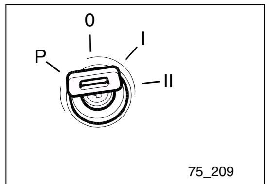
6. Release the ignition key as soon as the engine started. It automatically returns to the operating position 'I'.
