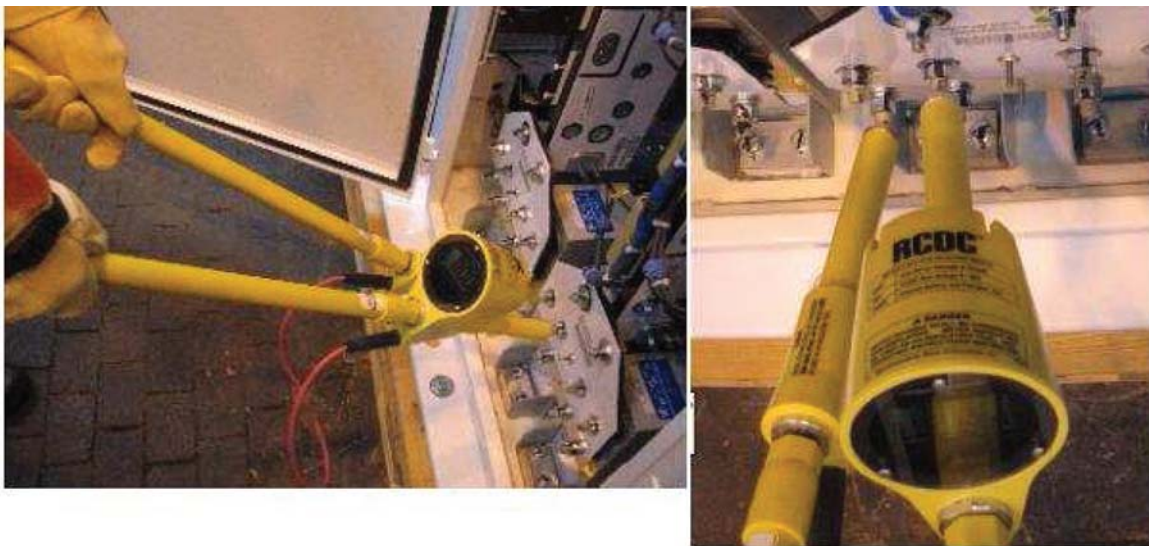
FIGURE 20-7. DC METER ON CAPACITOR
