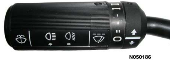
FIGURE 32-3. MULTI-FUNCTION TURN SIGNAL SWITCH
