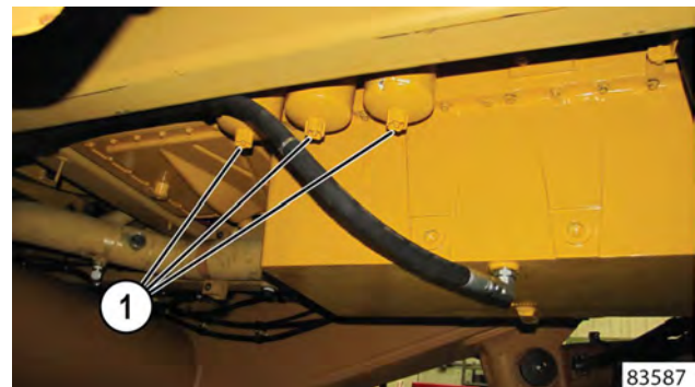
1. Water Drain Valves
