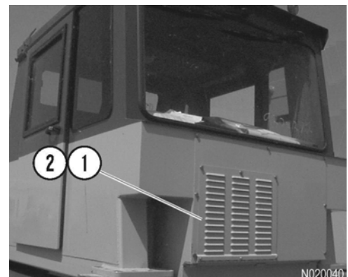
FIGURE 40-4. 1. Filter Cover 2. Cab Filter
