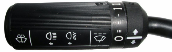
FIGURE 32-3. MULTI-FUNCTION TURN SIGNAL SWITCH
