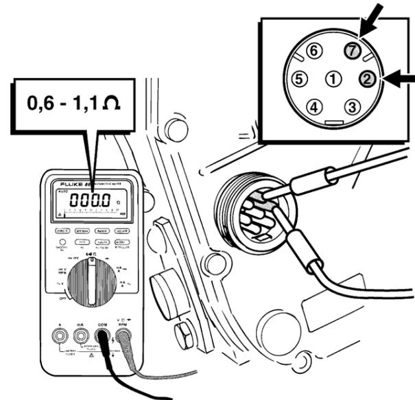
2. Use a multimeter to measure between pins 2 and 7. The multimeter should show 0.6 – 1.1 Ω.
