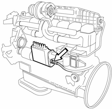
1. Undo the connector on the injection pump actuator.
