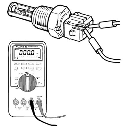
1. Undo the charge air temperature sensor connector.
