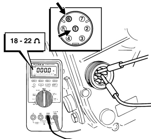
3a. Use a multimeter to measure between pins 1 and 6. The multimeter should show 18 -22 Ω.
