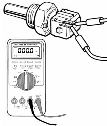
1. Undo the coolant temperature sensor connector.
