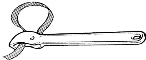
Tool for removing fuel and oil filter 99991796.
