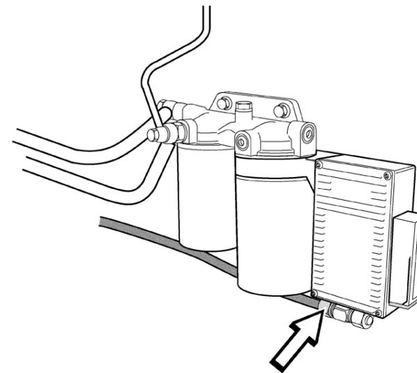
4. Undo the charge air pipe from the T-nipple underneath the control unit.
