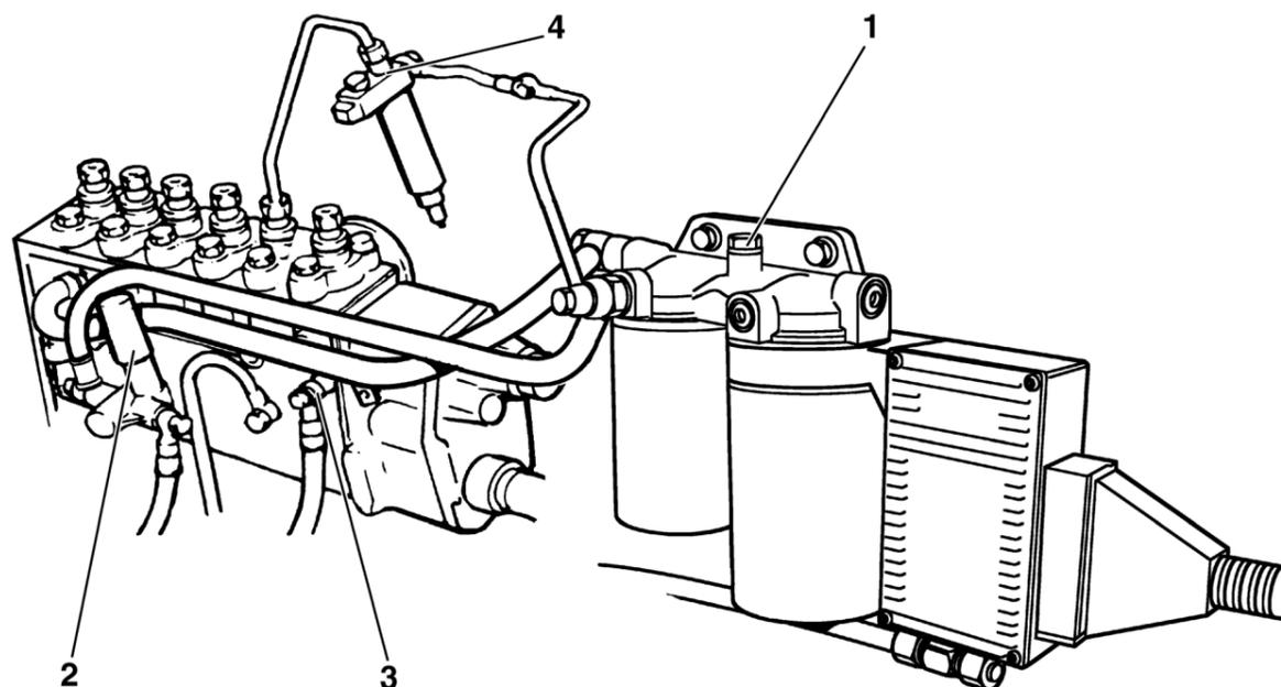
1. Vent screw on filter bracket
