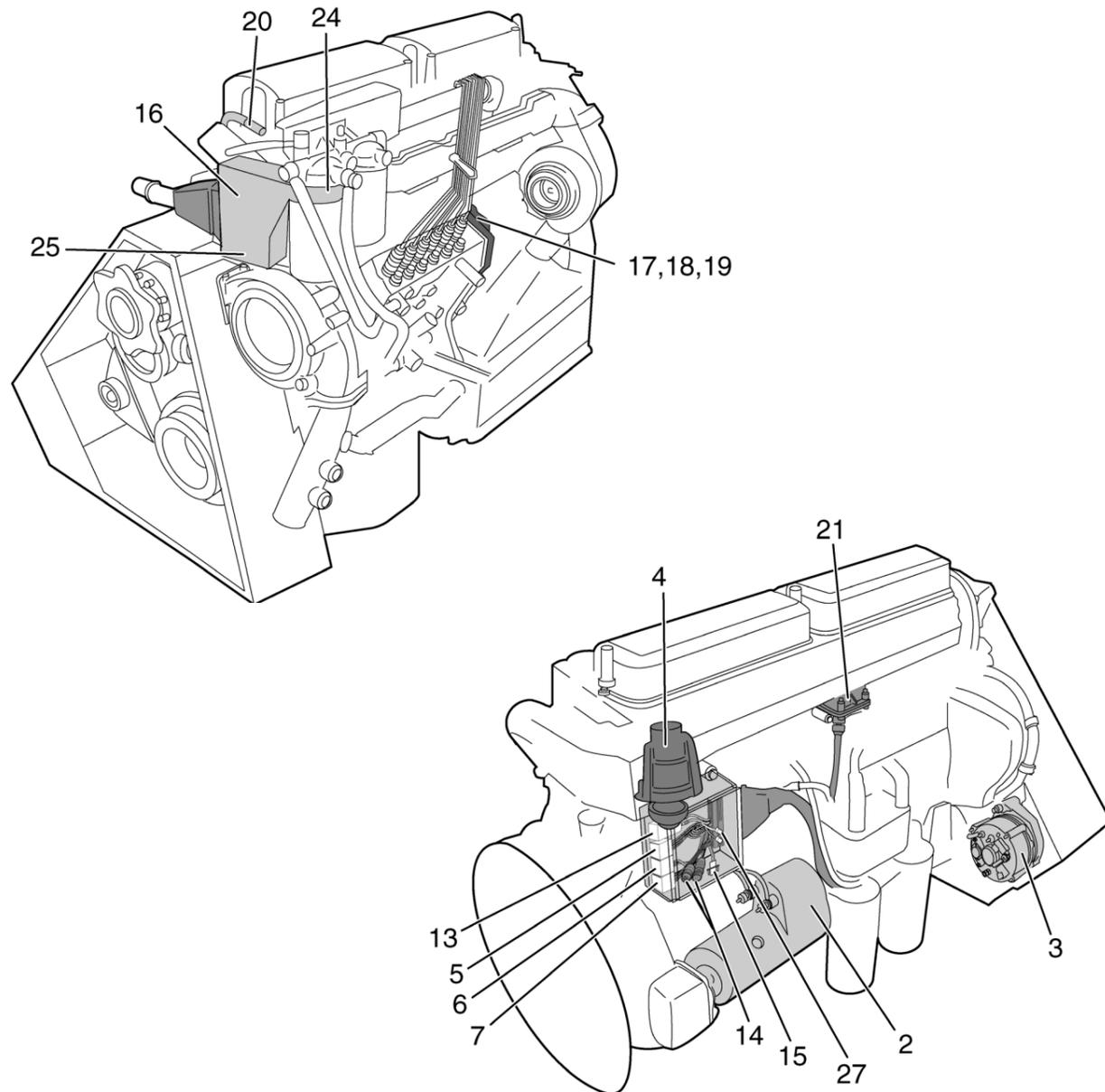
The positions in the illustration of the EDC system are the same as the positions on the wiring diagram, and show where each component is located on the engine.
