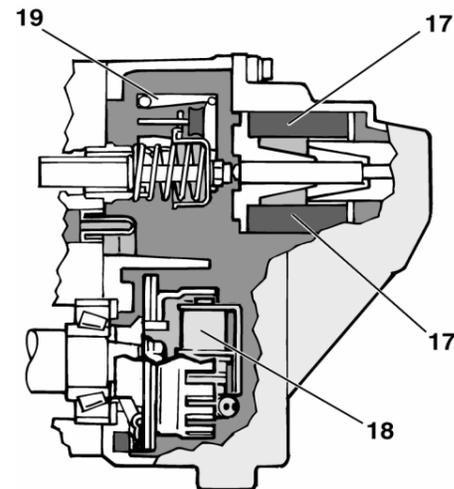
Electromagnetic actuator, EDC
