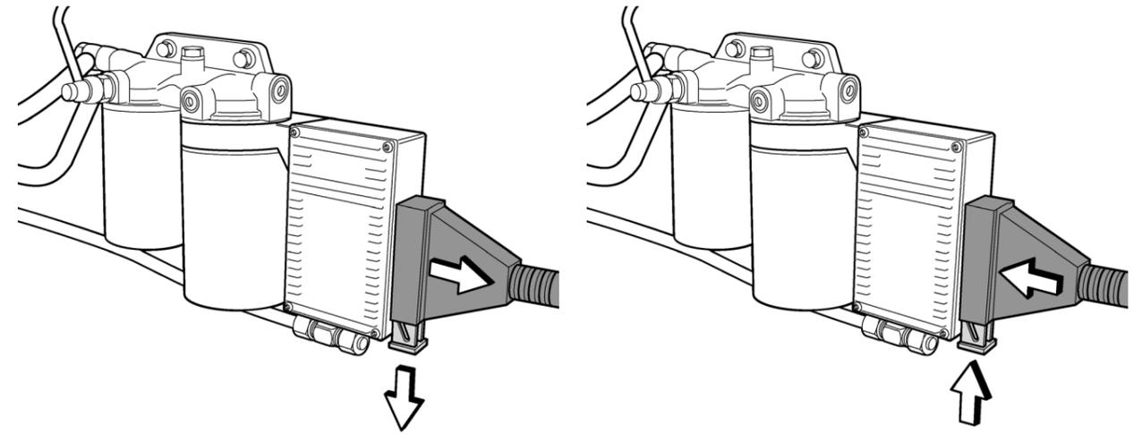
3. Pull the catch arm down at the same time as you pull the connector back.
