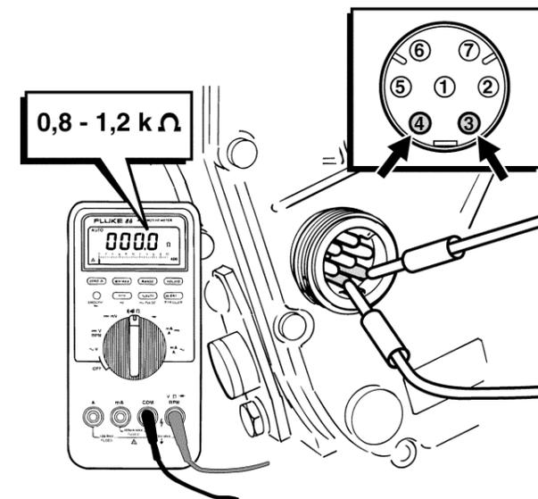
4. Use a multimeter to measure between pins 3 and 4. The multimeter should show 0.8 – 1.2 kΩ.
