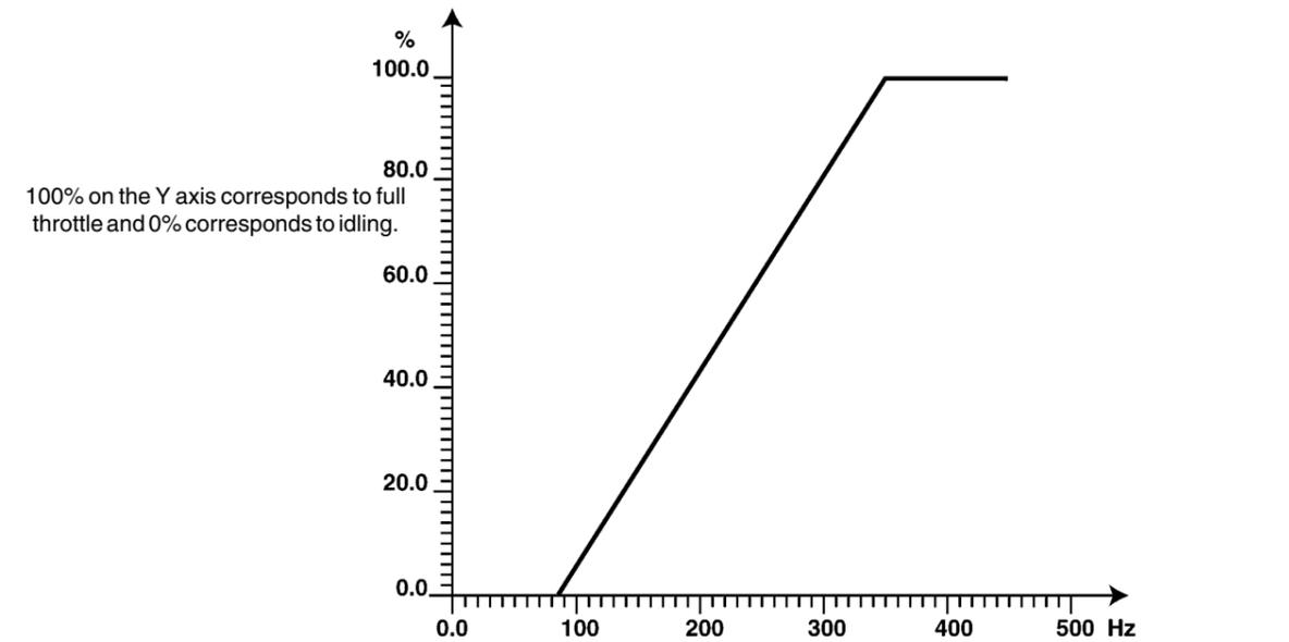
Frequency control. 85 Hz corresponds to idling and 350 Hz corresponds to full throttle.
