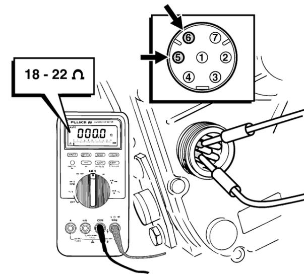
3b. Or use a multimeter to measure between pins 5 and 6. The multimeter should show 18 - 22 Ω.
