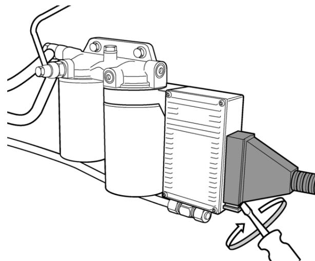
2. Remove the control unit connector, by inserting a screwdriver **between** the red catch arm and the connector. Turn the screwdriver to partly pull the catch arm out of the connector.
