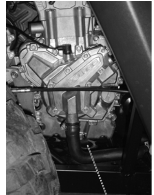
Drain Plug Access
