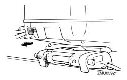
Insert the knotted end of the emergency starter rope into the notch in the flywheel rotor and wind the rope several turns around the flywheel clockwise.
