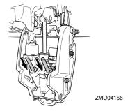
Activate the trim-up switch until the tilt rod is fully extended. Unlock the tilt support lever.
