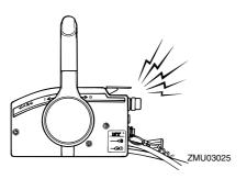
If the warning system has been activated, stop the engine and check for the cause.
