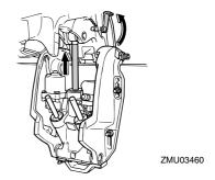
8. Tilt the outboard motor down. Check that the tilt rod and trim rods operate
