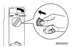
Immediately after the engine starts, release the main switch and allow it to return to "ON" (on).
