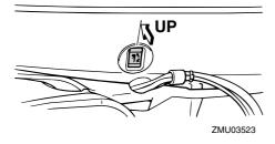
Push the tilt support knob into the clamp bracket or pull the tilt support lever toward you to support the engine.
