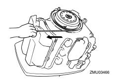
Give a strong pull straight out to crank and start the engine. Repeat if necessary.
