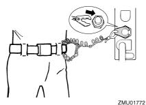
Turn the main switch to "ON" (on).
