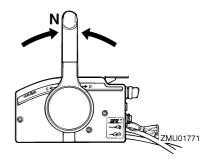
Slightly tilt the outboard motor up to the desired position using the power trim and tilt switch / power tilt switch.
