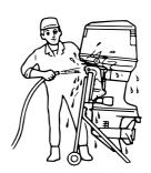
Remove the spark plugs and face the spark plug holes downward to allow any water, mud, or contaminants to drain.
