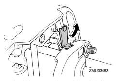
Push the power trim and tilt switch / power tilt switch "DN" (down) to lower the outboard motor to the desired position.
