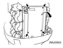
2. Disconnect the yellow cord (emergency circuit) of the CDI unit to return to port.
