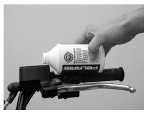
NOTE: To speed up the brake bleeding procedure, the master cylinder can be purged of air before brake line is attached. Fill with DOT-approved brake fluid and pump lever slowly two to three times with finger over the outlet end to purge master cylinder of air.
