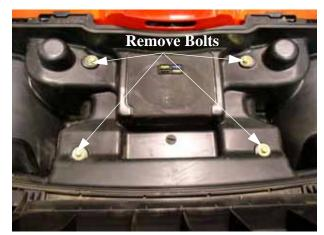
3. Remove the two (T25) screws that secure the storage box to the front fender well areas (each side).
