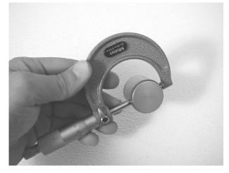
3. Inspect the brake disc and pads as outlined for brake pad replacement in this section. See "BRAKE PAD INSPECTION" earlier in this chapter.
