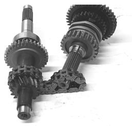
18. Remove the rest of the bearings from the shafts.
