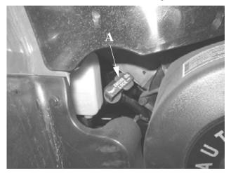
3. Unlock the lever lock (A). Remove dipstick (B) and wipe dry with a clean cloth.
