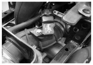
Air passing through the intake is measured by the T-BAP and relayed to the ECU. These signals, comprised of separate air temperature and barometric air pressure readings, are processed by the ECU and compared to it's programming for determining the fuel and ignition requirements during operation.
