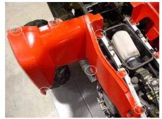
3. Reverse the removal procedures to install the quarter panels. Verify panels are properly aligned to the footwell end upon reassembly.
