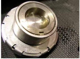
NOTE: Excessive debris in the oil and/or noise coming from the front drive on deceleration are key indicators of clutch pack failure. Replace clutch as an assembly if found to be worn or damaged.
