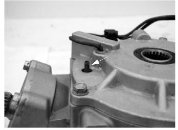
Using a 3/32 hex wrench, turn the back-lash screw out 3-4 turns. Re-apply Loctite 262<sup>™</sup> onto the bottom screw threads.
