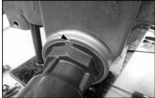
6. Install the output gear assembly. Be sure to properly mesh the snorkel shaft bevel gear with the output bevel gear. Install the 4 torx screws (2) to secure the output gear assembly into place. Torque screws to .
