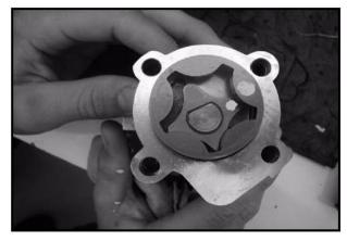
NOTE: If replacing the old rotors, new replacement rotors will fit into the old oil/water pump housing.
