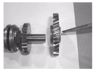
21. Remove the gear, split bearing, and washer from the reverse shaft.
