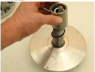
3. Inspect surface of shaft for pitting, grooves, or damage. Measure the outside diameter and compare to specifications. Replace the drive clutch assembly if shaft is worn or damaged.
