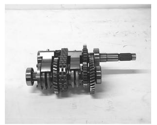
11. Remove the shift forks from the assembly. Note the correct position of each fork.
