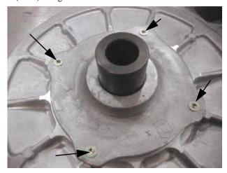
4. Place the clutch into Clutch Compression Tool **PN 8700220**. Using Compression Extensions **PN PS-45909**, Press down on top of the spider assembly, compressing the spider onto the shaft. Remove snap ring (A) and slowly release the assembly.
