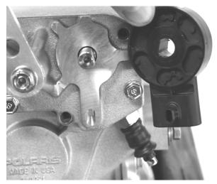
NOTE: Rotate the bellcrank to line the flat side of the switch up to the flat side of the shaft.
