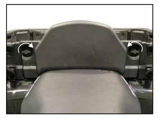
2. While pulling the backrest towards the front of the ATV, lift up on the passenger backrest loop that is face down in the cargo box.
