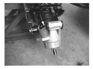
3. Pull sharply outward to remove shaft from transmission. Install a new compression ring upon assembly.
