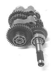
NOTE: Use caution when installing the fork, as the spring can easily fall out.
