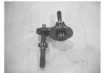
2. Install front and rear output shafts into the case.
