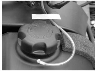
5. With all the body panels removed from the front of the ATV and the gas tank exposed, disconnect the pump wiring harness.
