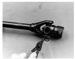
NOTE: If yoke or bearing is removed, cross bearing must be replaced. Note orientation of grease fitting (if equipped) and mark inner and outer yoke for correct re-positioning during installation.
