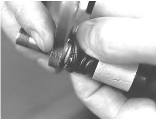
4. Compress the mounting bracket and make sure the dust seals are fully seated. Install the brake pads. Clean the disc and pads with brake parts cleaner or denatured alcohol to remove any dirt, oil or grease.
