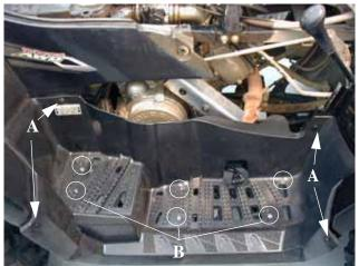
3. Reverse the removal procedures to install the foot well. Be sure to properly align the cab ends into the foot wells upon reassembly.
