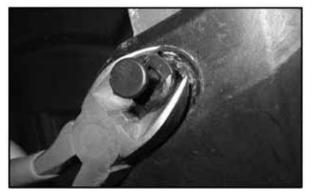
2. Remove the four screws (B) from the bottom of the foot well. Remove the footwell.
