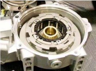
14. Install the remaining output clutch assembly. NOTE: Align locating pins / holes for installation.
