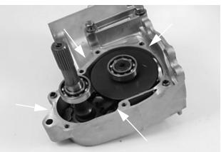
Apply Crankcase Sealant to mating surfaces.
