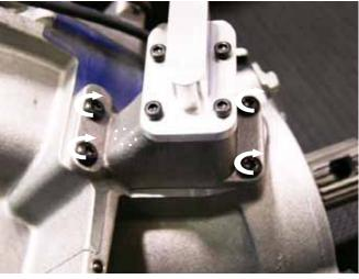
Ô = T Pump Assembly Screw Torque: 17-23 in. lbs. (1.9-2.5 Nm)
