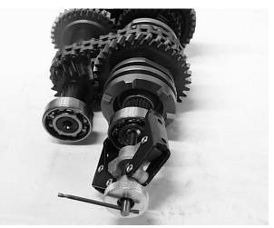
13. Remove the park lock engagement dog. Remove the wave spring and reverse engagement dog.
