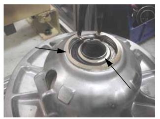
4. Line up the "X" on the moveable sheave with the "X" on the stationary sheave or use the marks previously used. Put the sheaves together.
