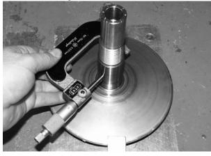
4. Visually inspect PTFE thrustwasher for damage. Measure the thickness and compare to specification. Replace if worn or damaged
