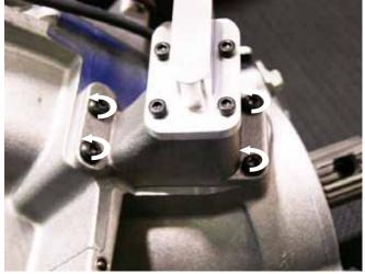
NOTE: Piston pump assembly is a non-serviceable item and should not be disassembled. Replace as an assembly if found to be damaged or non-working.
