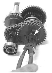
16. Remove low gear (33T) and the needle bearing.
