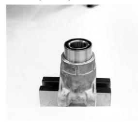
3. Press bearing into place until outer race bottoms on housing.
