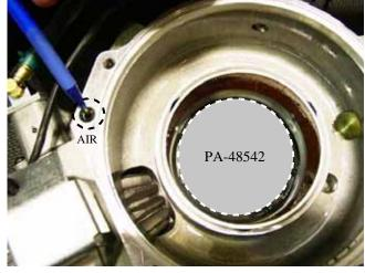
3. Remove and discard the inner and outer o-rings from the piston assembly.
