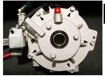
4. Remove the outer cover plate assembly. Remove and inspect the cover o-ring (1). Inspect thrust bearing (2) for wear. Replace items as required.
