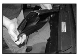
To install the front cover place top lip of the cover into and lift up to remove.
