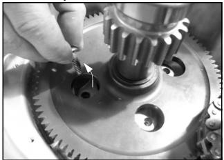
4. Assemble the input shaft assembly if previously disassembled.
