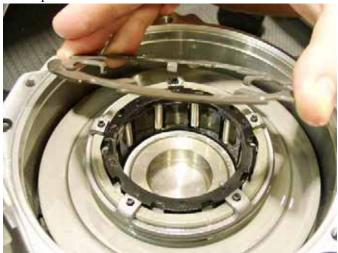
7. Remove the spacer. Inspect for signs of wear or damage. Replace component as required.
