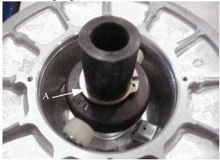
15. Install the cam assembly (helix) over the shaft. Line up the "X" on the cam, "X" on spider, and "X" on the stationary sheave or use the marks previously made before disassembly. **NOTE:** If the cam assembly (helix) is difficult to install, be sure the sheaves are aligned. To align the sheaves place the clutch assembly on a flat surface with the cam assembly (helix) side down. Press down on the moveable sheave belt face with both hands and the helix will release.
