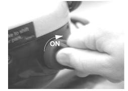
3. The word "Wait" will appear, the EFI module is now searching for blink codes. If any blink codes are stored they will display in numerical order on the instrument cluster.
