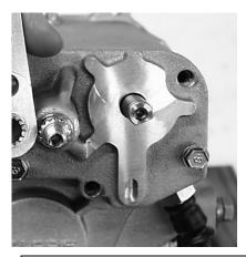
Torque Bellcrank Nut: 12-18 ft.lbs. (16-24 Nm)
