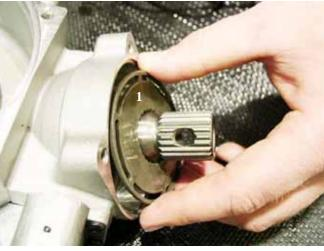
7. Install the input shaft cover assembly, bolts and bracket. Torque to specification.
