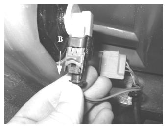
2. To remove the brake light electrical connector (B), press in on the tab on the connector to unlock the connector and pull the connector from the bulb assembly.
