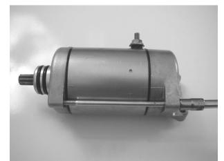
Install the starter onto the engine case. Hand tighten each of the starter bolts. Torque the bottom bolt first to 9 ft.lbs. (12 Nm). Then torque the top bolt to the same specification.
