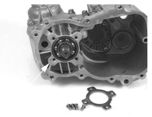
26. Remove the front housing cover screws.
