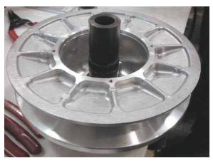
5. Install the roller (A) onto the roller pin (B). (Both Sides).
