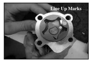
18. Apply assembly lube or oil to the rotors on the oil pump shaft.
