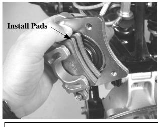
If the brake pads are contaminated with grease, oil, or liquid soaked do not use the pads, use only new clean pads.
