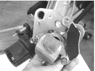
7. Measure the thickness of the pad material. Replace pads if worn beyond the service limit.
