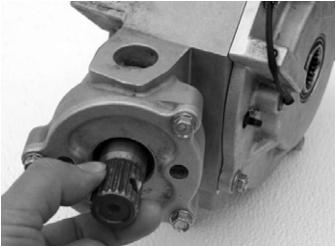
5. If a tight spot is felt during rotation, loosen the backlash screw another 1/8 turn. Perform the step 16 again. Repeat this procedure until the pinion shaft rotates smoothly 4 times (1 revolution of ring gear).
