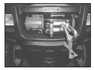
The mini-rocker (IN/OUT) control controls the direction of the cable for the winch. IN pulls the cable into the winch and OUT feeds the cable out of the winch.
