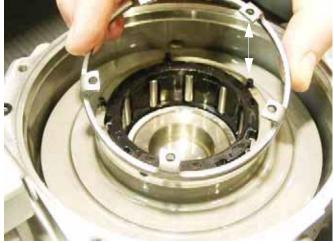
12. Install the armature plate. Verify the armature plate tabs align with tab recesses in the roll cage.
