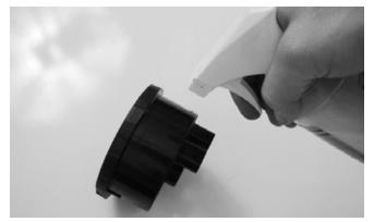
2. Be sure the rubber grommet inside the pod is fully installed and that the indexing key is in the headlight pod keyway.
