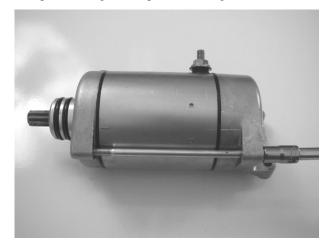
NOTE: Note the alignment marks on both ends of the starter motor casing. These marks must align during reassembly.
