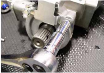
Input Cover Bolt Torque: 7-11 ft. lbs. (9.4-14.9 Nm)
