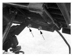
8. Support the cargo box and remove the clip and pin holding the gas shock to the cargo box.
