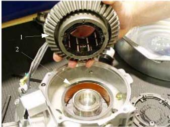
9. Remove and inspect the bearing surfaces of the output hub.
