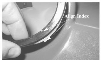
3. Hold the pod assembly securely and insert the instrument cluster into the pod assembly. Twist the instrument cluster gently in a clockwise motion to properly seat the instrument cluster into the pod assembly. Apply pressure on the bezel while pressing down on the instrument cluster.
