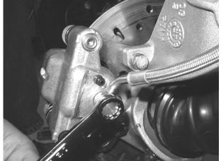
2. Push upper pad retainer pin inward and slip brake pads past edge. Loosen pad adjuster.
