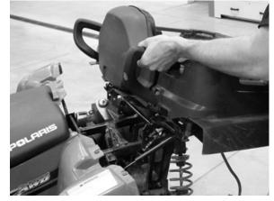
10. Reverse the removal steps to reinstall the cargo box. Refer to the standard fastener torque values in Chapter 1 during assembly.
