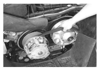
4. Measure belt width and replace if worn. Generally, belts should be replaced if clutches can no longer be adjusted to provide proper belt deflection.
