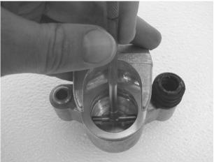
2. Inspect piston for nicks, scratches, wear or damage. Measure diameter and replace if damaged or worn beyond service limit.
