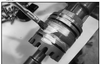
5. Install the snorkel shaft assembly into the gearcase. Install the snorkel shaft assembly in until the second O-ring is contacting the gearcase, but is still visible.
