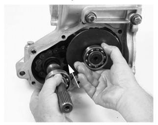
3. Before installing the cover make sure the sealing surfaces are clean and dry, and shafts are fully seated in the transmission case. Apply Crankcase Sealant (**PN 2871557**) to the mating surfaces.
