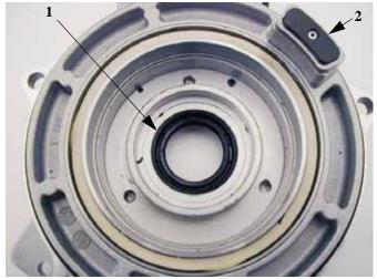
NOTE: Ring gear backlash (2) is set at the factory. No adjustment is required, unless the front cover is replaced or the back lash pad screw is removed.
