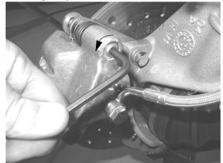
4. Remove caliper from mounting bracket.
