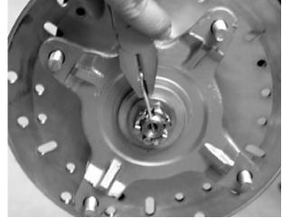
4. Install hub and tighten hub nut to specification.
