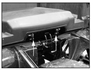
2. Remove the two pivot pins holding the seat bottom to the frame and then lift up on the seat bottom to remove.
