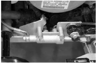
1. Remove the RH footwell to gain access to the rear master cylinder.
