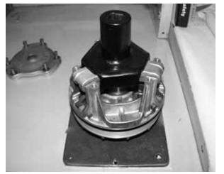
ClutchHoldingFixture: (PN 2871358) Spider Removal Tool: (PN 2870341)
