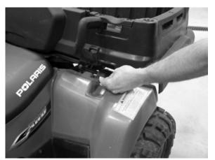
7. Remove the four bolts attaching the rear of the cargo box to the frame. There are two on each side.
