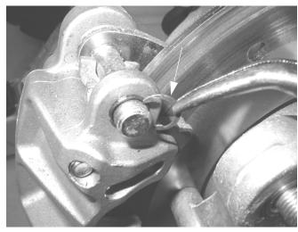
3. Loosen the slide pins with a hex wrench.
