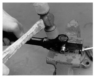
4. Force U-joint cross to one side and lift out of inner yoke.
