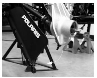
10. Pull strut assembly out while pivoting front drive shaft downward until it clears strut assembly.
