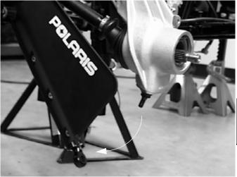
6. Pull the hub and strut assembly out and pull the drive-shaft out of the hub.
