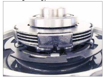
15. Place cover assembly on Install bolts (arrows) retaining the outer cover plate assembly and torque to specification.
