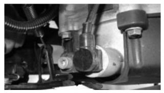
$\begin{array}{l} Crankshaft Position Sensor Gap: \\ .059'' \pm \ .010 \ inch \\ (1.0 \pm .26 \ mm) \end{array}$
