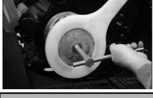
**Drive Clutch Puller:** (PN 2870506) **Clutch Holding Wrench:**
