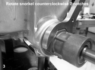
2. Once the gear backlash is found, to install the snorkel lock screw, you may have to rotate the snorkel tube clockwise or counterclockwise slightly. This will allow the lock screw to thread itself into one of the slots of the snorkel tube (See illustration below) to secure the snorkel tube.
