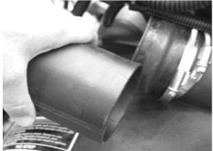
4. Remove the gas tank cover vent hose. Be sure to properly route the vent hose upon reassembly.
