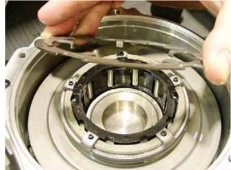
13. Install new cover o-ring (1) on the cover plate assembly and a new passage o-ring (2) on the gear case.
