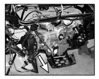
NOTE: Use caution when lifting the engine out of frame. Use an engine lift or other means if the engine is too heavy to be lifted manually.
