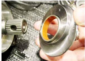
6. Install the splined armature plate (1).
