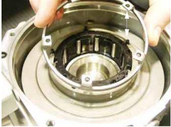
8. Remove the ring gear (1) and spacer (2).
