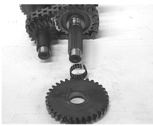
17. Remove the reverse gear shaft.
