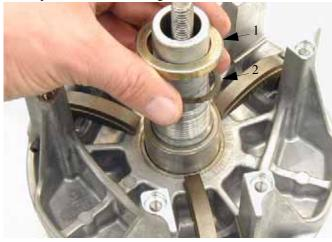
Thrust Washer Thickness Standard: .030, (.76mm) Service Limit: .025, (.64mm)
