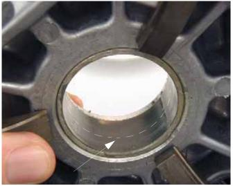
Moveable Sheave Bushing Inspection: Replace the cover bushing if more brass than Teflon™ is visible on the bushing. Refer to bushing replacement in this chapter.
