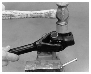
3. Support U-joint in vise as shown and drive inner yoke down to remove remaining bearing ca
