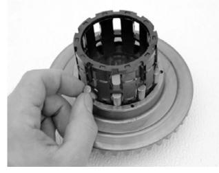
10. Install the clutch pack (1), spacer (2) and ring gear (3). **NOTE: Align locating pins / holes for installation.**
