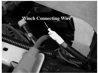
The Orange/White wires are located under the front cover (under headlight pod). The Orange/White wires supply the control power to the winch.
