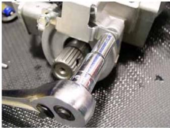
16. Inspect the magnetic coil (1) and bushing in the input cover plate assembly. Replace the input cover seal.
