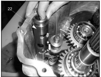
17. Remove the output gear (21) and gear cluster assembly from the gearcase by pulling both assemblies straight up. Place the gear cluster assembly on a clean surface for inspection.
