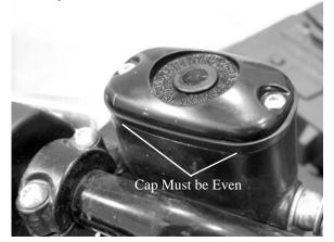
14. Torque the screw to specification .
