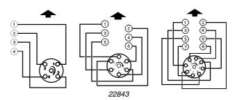
Spark plug wires must be arranged between the distributor cap and spark plugs in the order of firing sequence. If spark plug wires are not correctly installed, misfiring or cross-firing will result.
