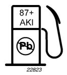
EFI models: Some marinas sell fuel with lead additives. Do not use leaded fuel, as it may block the fuel injectors and cause leakage.
