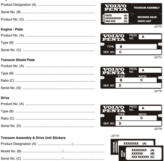
**NOTE!** The Transom Assembly & Drive Unit Stickers shown above should be located on the Engine Decal. Your Volvo Penta dealer will have attached these stickers at the time that the transom assembly and drive unit were mounted on your boat and attached to the engine.
