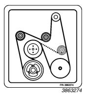
The label depicting the serpentine belt configuration is typically mounted on a flat surface located on the side of the alternator/automatic tensioner bracket or on the power steering pump/reservoir.
