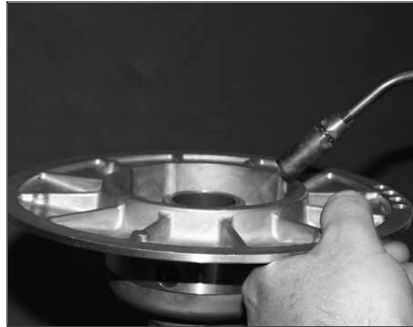
Heat Bushing Surface Prior To Installation/ Removal OF Bushings
