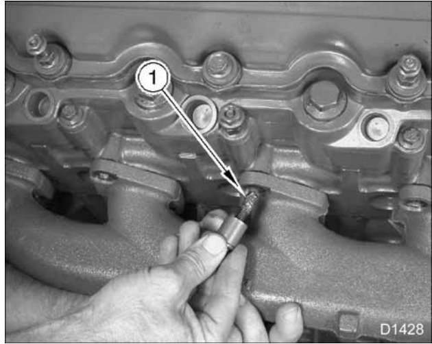
Figure 124 Bolt and spacer for left exhaust manifold
