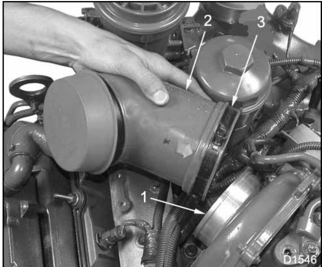
Figure 50 Air inlet duct
