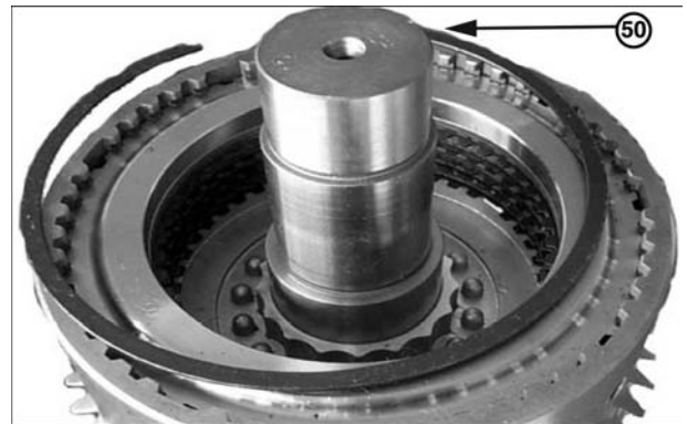
19. Using a screw driver, disassemble snap ring (50) from cylinder.
