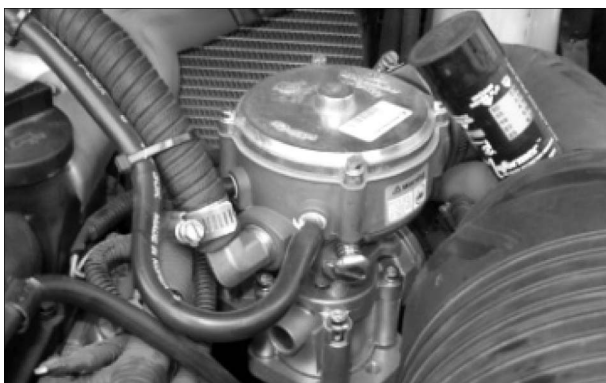
Figure 11. CA100 Mixer Installed with Electronic Throttle
