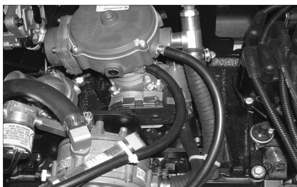
Figure 11. CA100 Mixer Installed with Electronic Throttle
