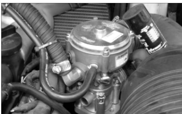
Figure 11. CA100 Mixer Installed with Electronic Throttle
