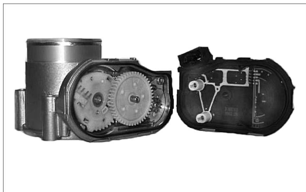
Figure 18. Throttle Position Sensor (TPS) on DV-E5 Throttle
