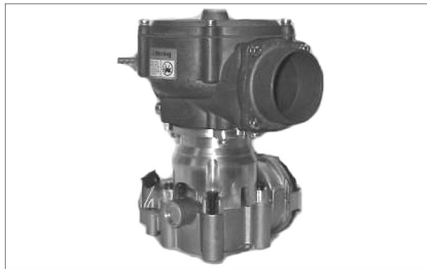
Figure 8. CA100 Mixer Attached to Throttle Body
