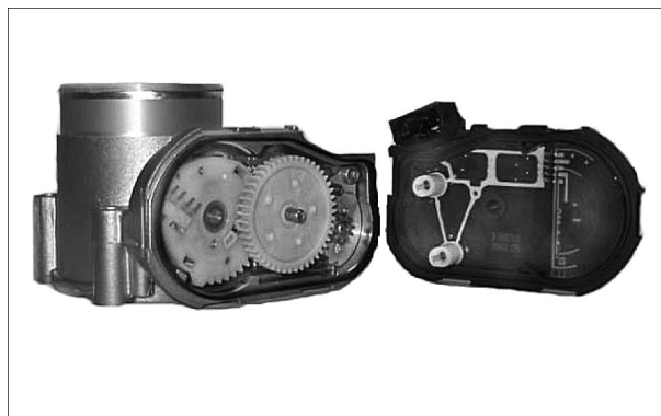
Figure 20. Throttle Position Sensor (TPS) on DV-E5 Throttle
