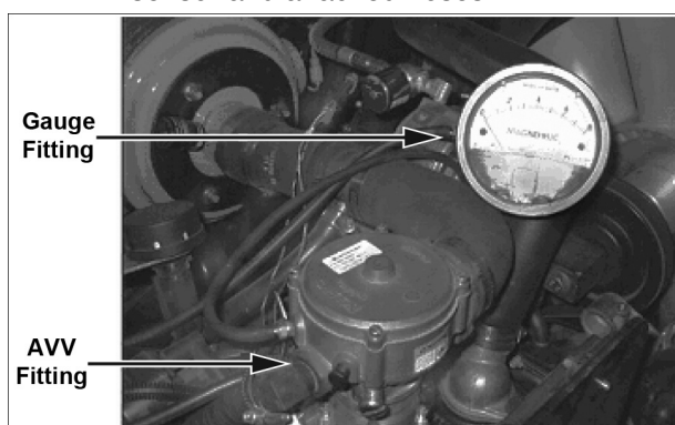
Figure 37. Magnehelic Gauge Connection
