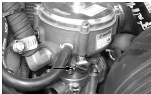
Figure 12. Idle Mixture Adjustment Screw
