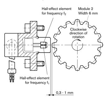
The frequency signals can only be evaluated in the measuring range from 2 Hz to 6 kHz.
