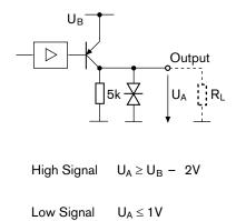
The output circuits for the speed signal and direction of rotation signals are indentical.
