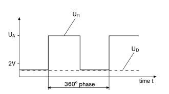
The frequency signal and direction of rotation signal can only be evaluated in the measuring range from 2 Hz to 6kHz.
