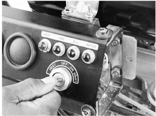
Starting Engine Using Key Switch (Earlier Engines)
