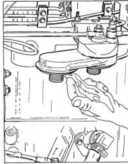
Fig. 5.31. Cleaning Fuel Filter Header
