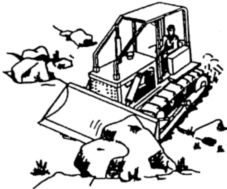
Fig. 4.42. Loosening Rocks with Lower Edge of the Blade
