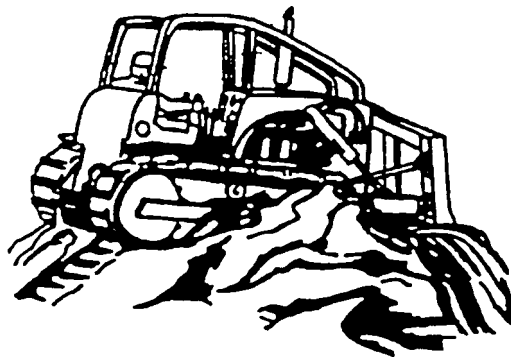
Fig. 4.34. Slope Edge Operation
