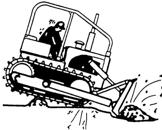
Fig. 4.29. Moving Material Downgrade
